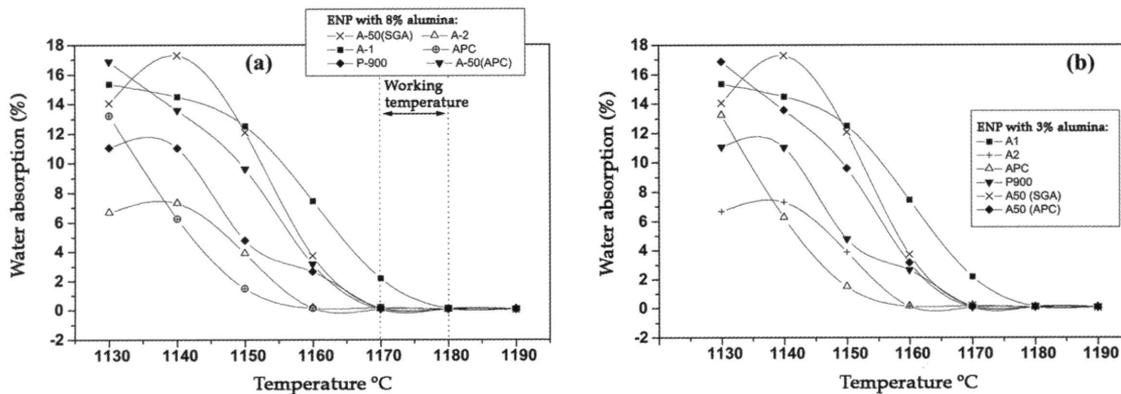
Figure 2. Behaviour based on firing temperature: (a) water absorption of ENP, containing 8% of different aluminas and (b) shrinkage of the height of ESO test specimens containing different alumina APC contents.
