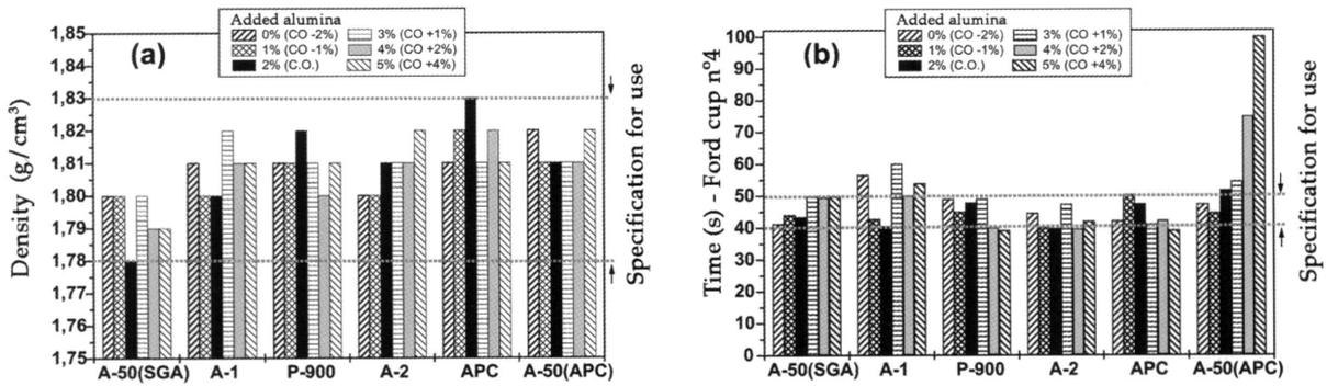
Figure 1. (a) Densities and (b) draining time of the ESO suspensions prepared with different aluminas.
