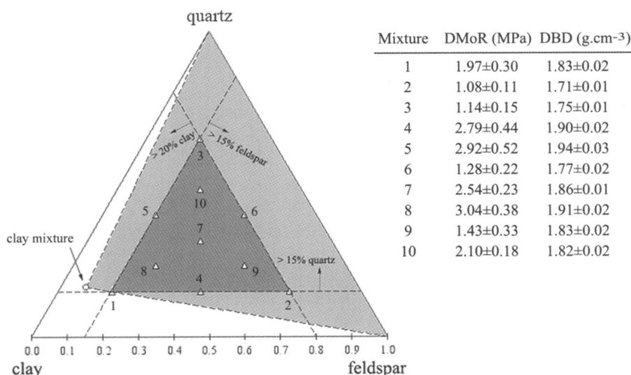
Figure 1. The ternary system clay-quartz-feldspar, showing: the raw materials triangle, the restricted pseudo-components triangle and the simplex points, and the measured values of DMoR and DBD.
