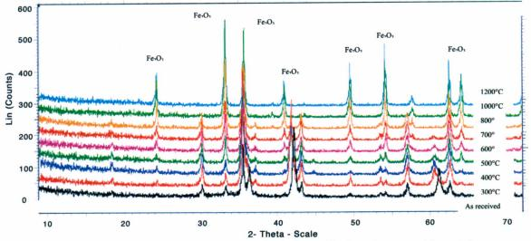
Figure 1. XRD at different calcination temperatures for the iron oxide pigments processed from steel scraps.
