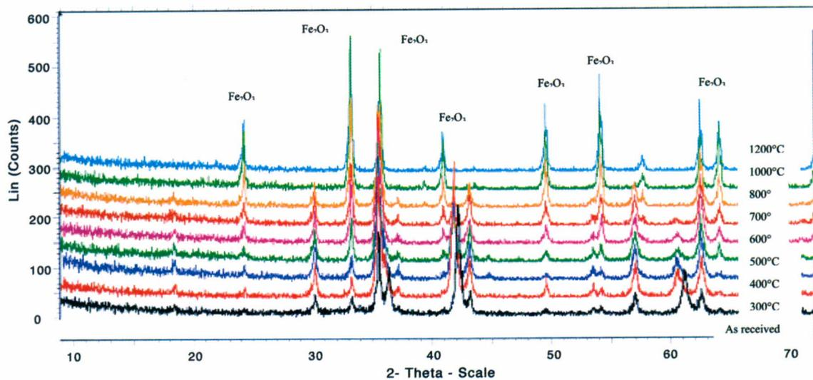
Figure 1. XRD at different calcination temperatures for the iron oxide pigments processed from steel scraps.
