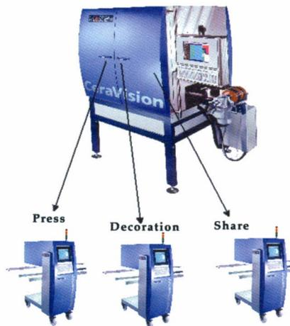
Figure 1. A family of small and low-cost before-the-kiln inspection systems have been derived from the automatic tile sorter
