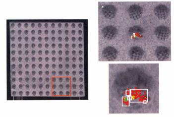
Figure 2. Defects in the embossing patterns are detected after the press
