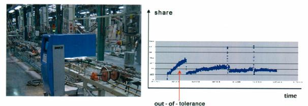
Figure 4. The stability of colour shade is monitored on the non-fired tiles
