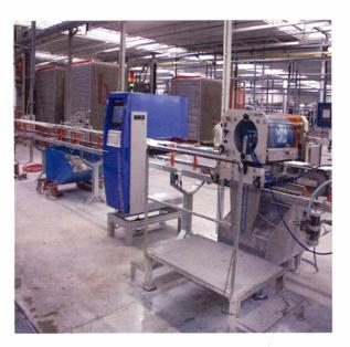
Figure 3. A screen printer is monitored for defects in the decoration pattern
