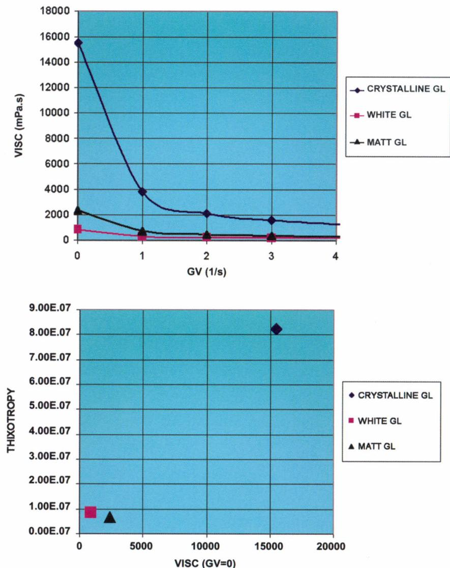
Figure 8 and 9. Comparative curves of rheological behaviour between different glazes.
