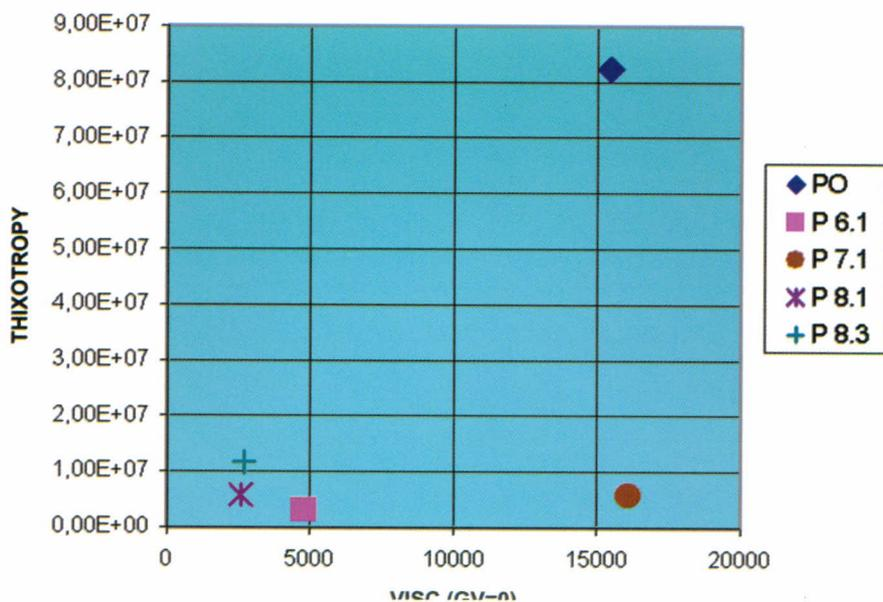
Figure 11. Thixotropy versus maximum viscosity at low shear rates.
