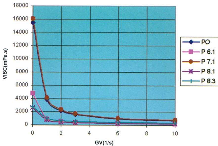
Figure 10. Rheological curves at low shear rates
