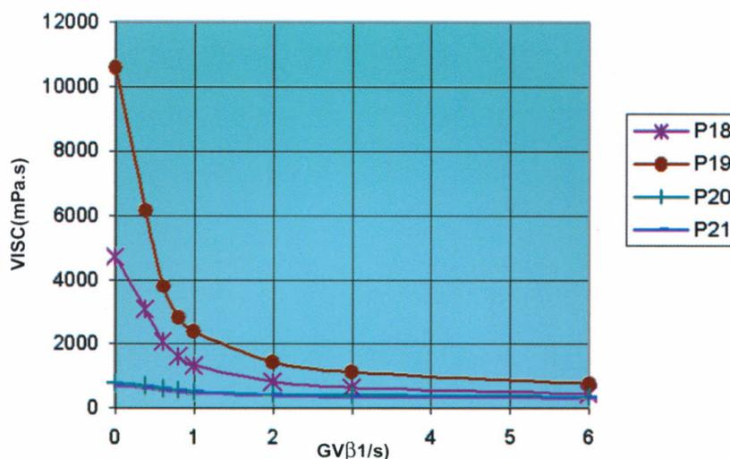
Figure 4. Rheological curves at low shear rates.
