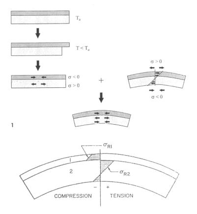
Figure 1. Residual stress profile originating from the TEC difference of the two layers
