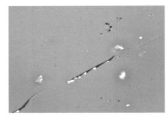
*Figure 14. SEM picture related to cracks observed in the glaze surface of tile with thick glaze after the autoclave test.*
