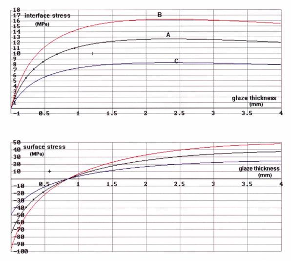
*Figures 9, 10. Residual stress at the interface and glaze surface for different glaze thicknesses of tiles for three different applied glazes.*
