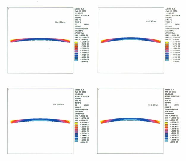
Figure 5. FEM results related to the curvature of tiles with different glaze thickness
