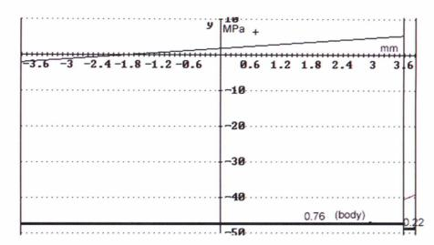
Figure 7. Residual stress profile in the specified glazed tile (according to the Timoshenko model)
