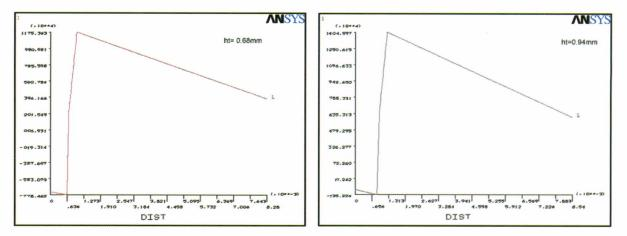
Figure 11. Residual stress profile in tiles with different glaze thicknesses (according to FEM)
