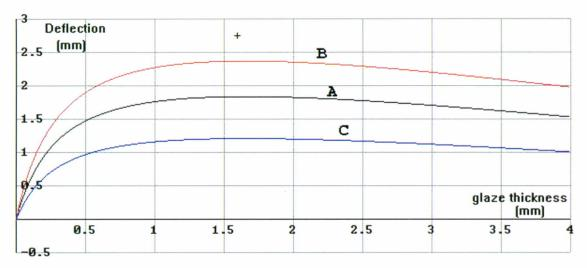
Figure 6. Glazed tile curvature versus glaze thickness (according to the Timoshenko model)
