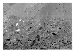
Figure 12. SEM picture of the glazed tile cross section showing cracks in the engobe layer (100 microns)
