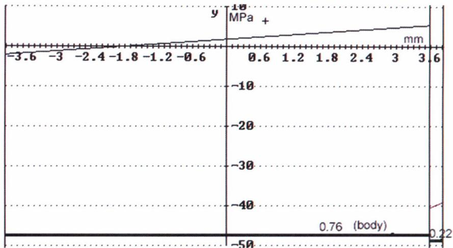
Figure 7. Residual stress profile in the specified glazed tile (according to the Timoshenko model)
