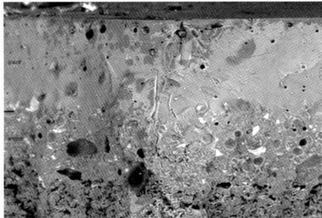
Figure 13. SEM picture of the glazed tile cross section showing cracks in the engobe layer (200 microns)
