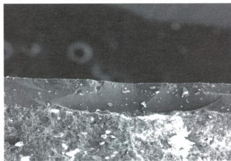
Figure 8. SEM picture of the glazed tile fracture section
