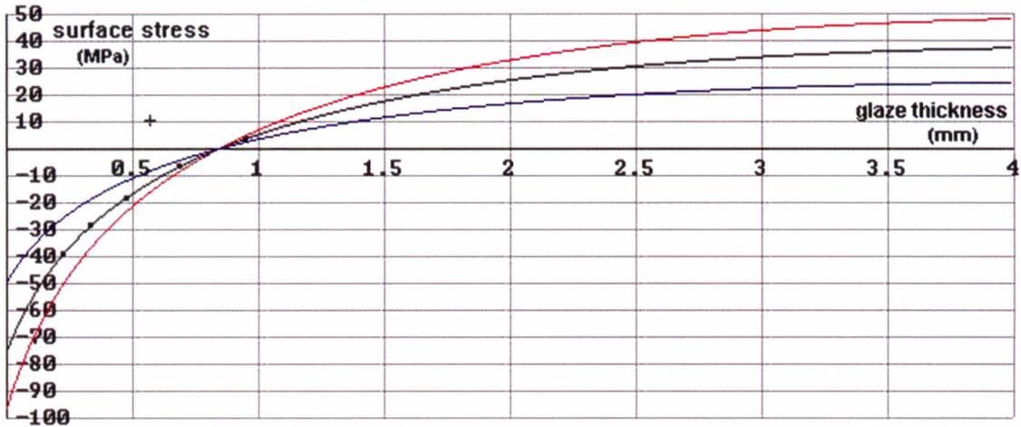
Figures 9, 10. Residual stress at the interface and glaze surface for different glaze thicknesses of tiles for three different applied glazes.
