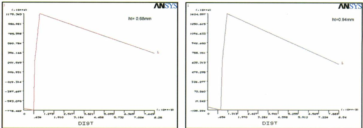
Figure 11. Residual stress profile in tiles with different glaze thicknesses (according to FEM)
