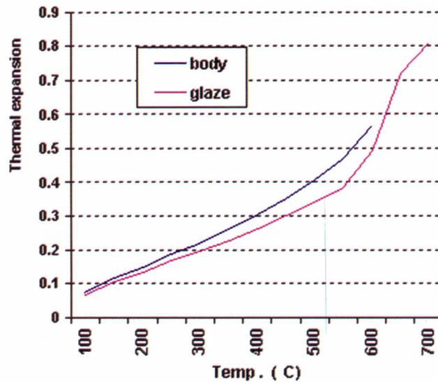
Figure 4. Dilatometric curve of body and glaze (A)
