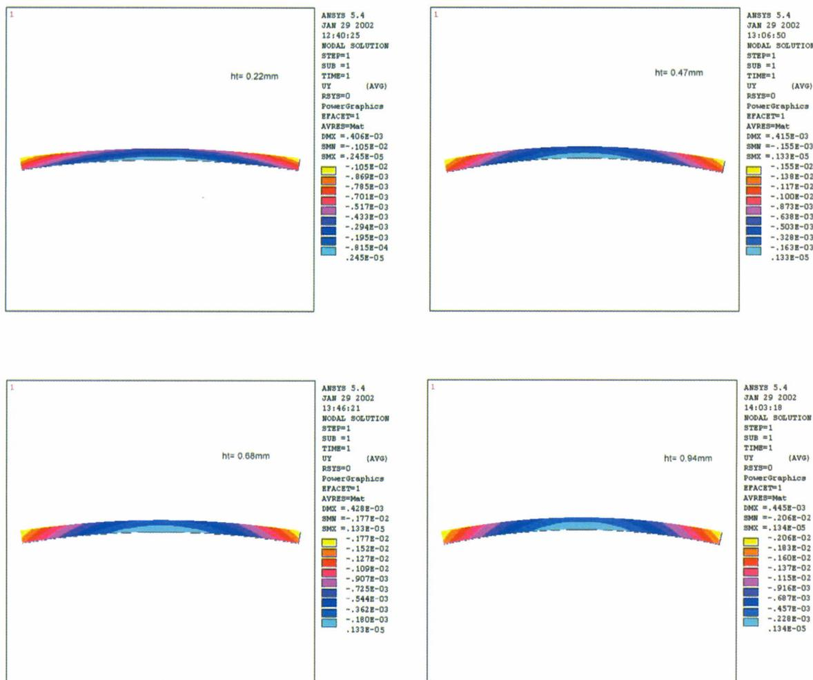
Figure 5. FEM results related to the curvature of tiles with different glaze thickness
