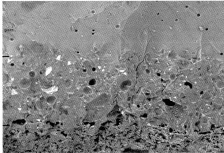
Figure 12. SEM picture of the glazed tile cross section showing cracks in the engobe layer (100 microns)
