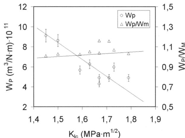
Figure 9. Influence of toughness on tile specific wear rate
