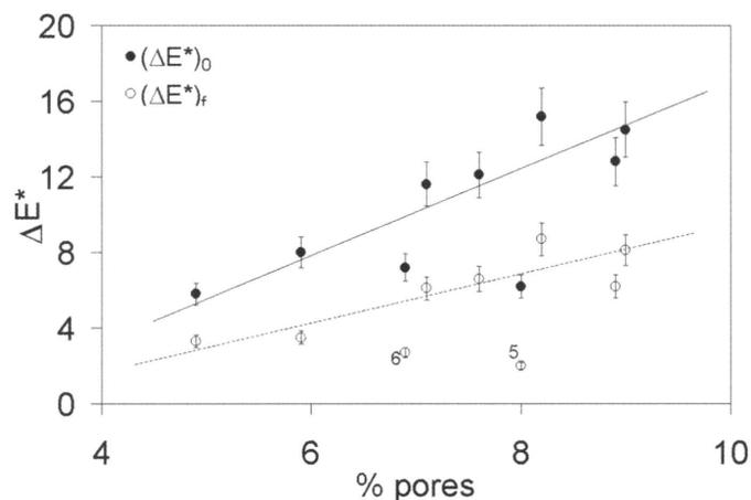
Figure 8. Influence of porosity on initial and final stain retention
