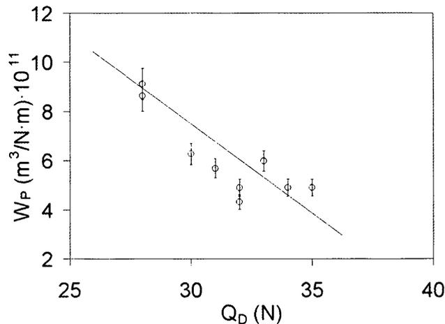
Figure 10. Influence of parameter  $Q_D$  on tile specific wear rate ( $W_p$ )
