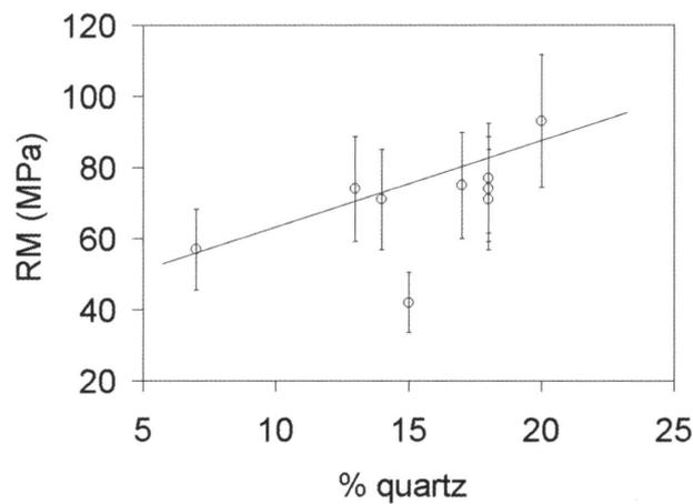
Figure 4. Influence of quartz content on mechanical strength
