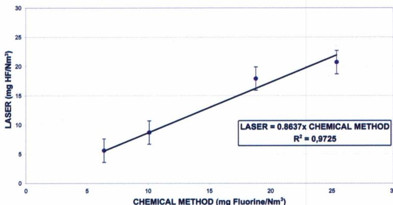
Figure 4. Correlation between the values of the LASER instrument and the standard chemical method.
