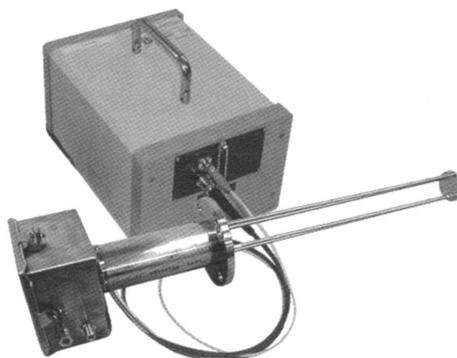
*Figure 3. Photograph of the LASER equipment: probe control unit and final configuration.*
