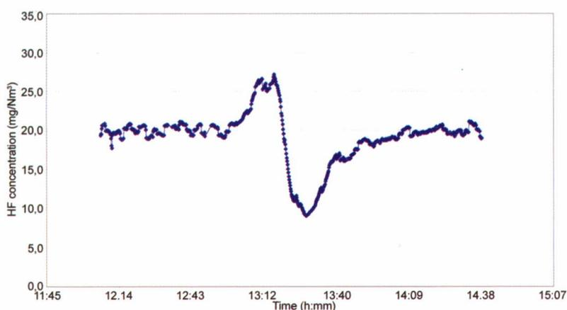
Figure 6. Evolution of the HF concentration on implementing modifications in the kiln.
