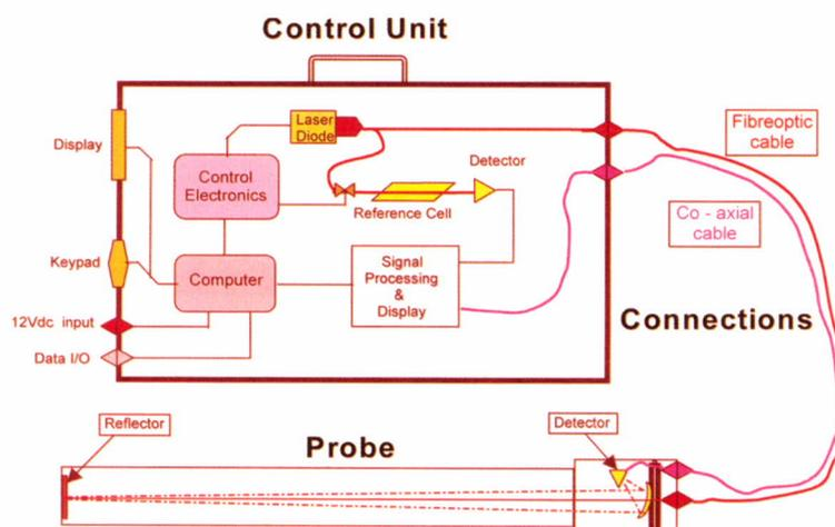
Figure 1. Schematic illustration of the equipment used.
