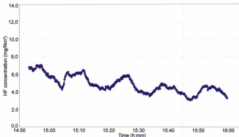
Figure 7. Evolution of the HF concentration on implementing modifications in the gas treatment system.
