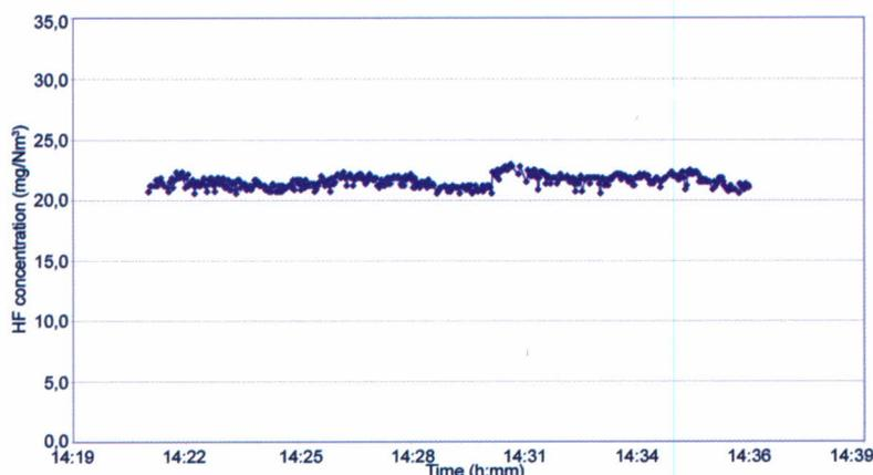
Figure 5. Example of the evolution of the HF concentration under standard operating conditions.
