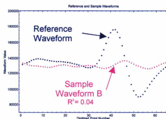
Figure 2b. Comparison of reference cell and sample B signals.
