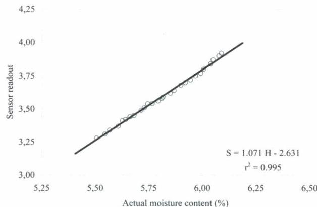
Figure 5. Relation between body moisture content and sensor readout
