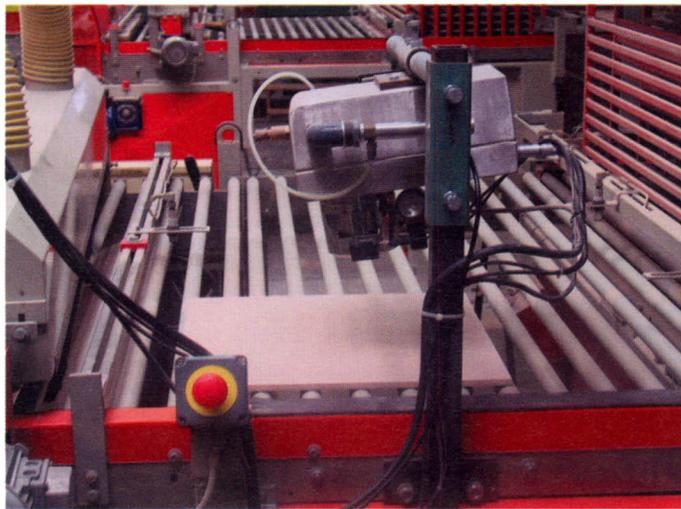
*Figure 6. View of the tile body moisture measuring equipment in the production line*
