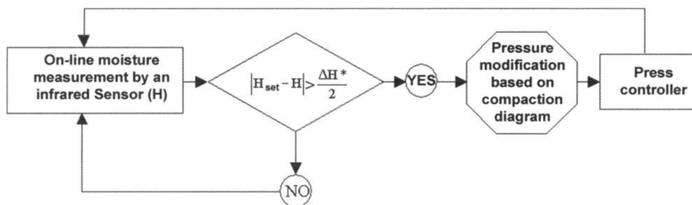
Figure 12. Schematic illustration of the proposed automatic pressing operation control
