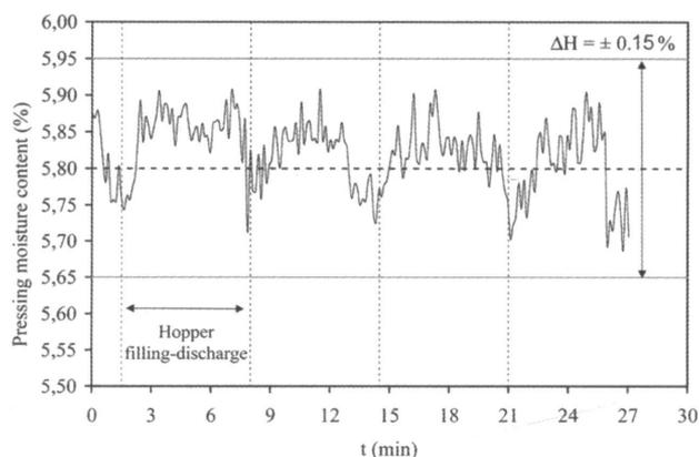
Figure 10. Moisture variations due to hopper filling cycles
