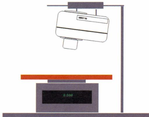
Figure 4. Measurement of body moisture content under static conditions
