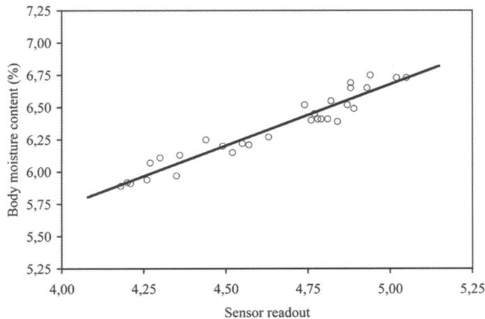
Figure 7. Calibration of the infrared moisture sensor
