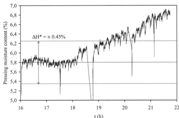
Figure 11. Evolution of pressing powder moisture in conditions producing calibers
