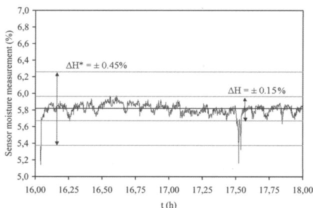
Figure 9 Evolution of freshly pressed tile moisture content
