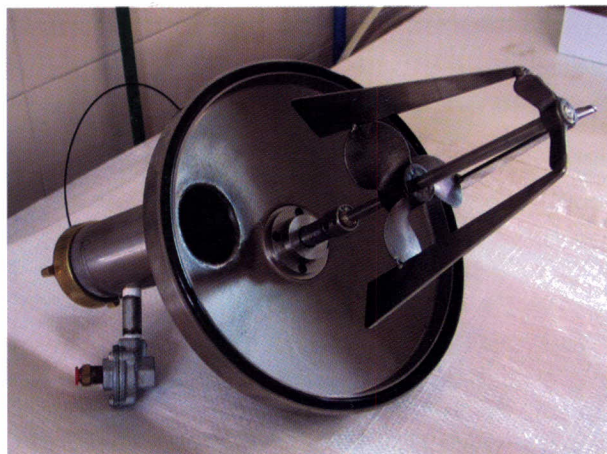
Figure 4. Detail of the tank lid and mixing blades
