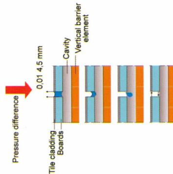
Figure 6: Water infiltration caused by pressure difference due to narrow joints (UAF, 2000)
