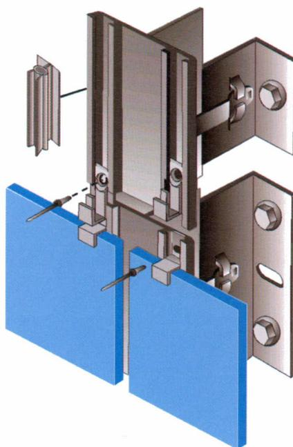
Figure 8: Visible coupling system (MIRAGE ENGINEERING, s.d.)
