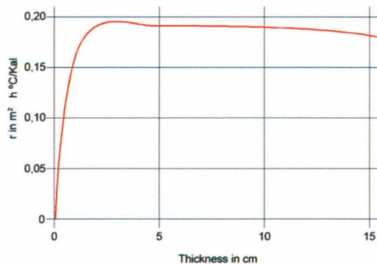
Figure 3: Cavity efficiency in terms of thickness (CROISET, 1970).
