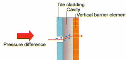
Figure 7: Water infiltration due to leaky cladding and faulty construction (UAF, 2000)
