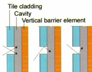
Figure 5: Water penetration caused by the droplet effect (UAF, 2000)
