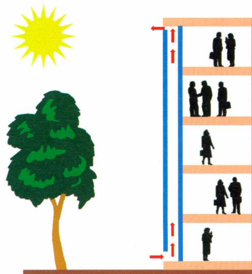
Figure 4: Cavity functioning scheme (CSTB, 2000)
