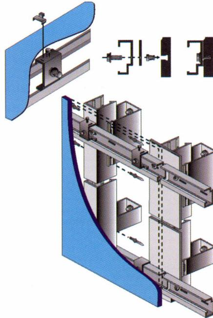
Figure 9: Non-visible securing system (MIRAGE ENGINEERING, s.d.)
