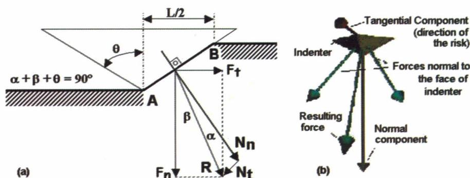
Figure 2. Forces acting in (a) general and (b) pyramidal indenter
