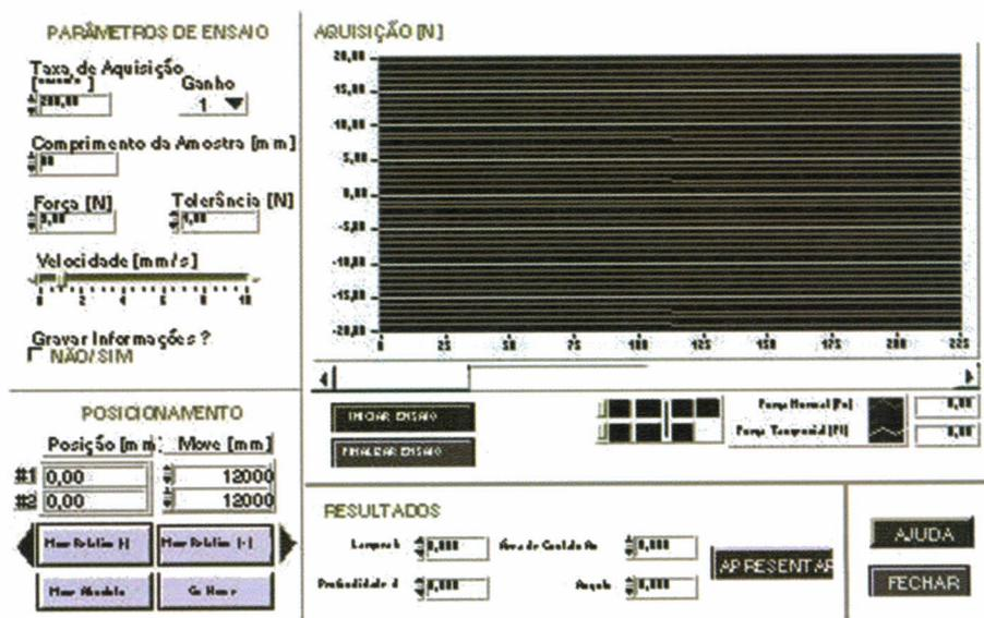
Figure 4. Software interface of the sclerometer
