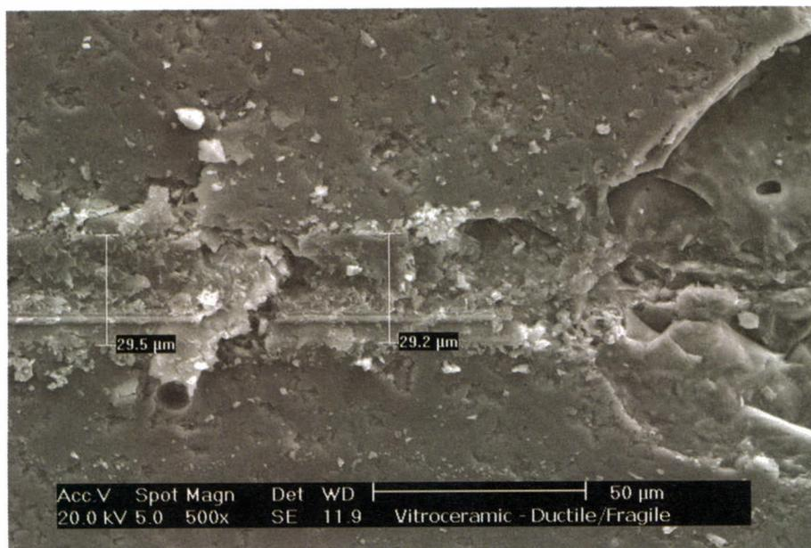
Figure 10. Ductile/brittle transition of the scratch in the glass-ceramic tile
