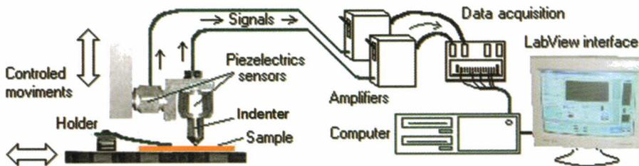
Figure 3. Schematic illustration of the sclerometric apparatus
