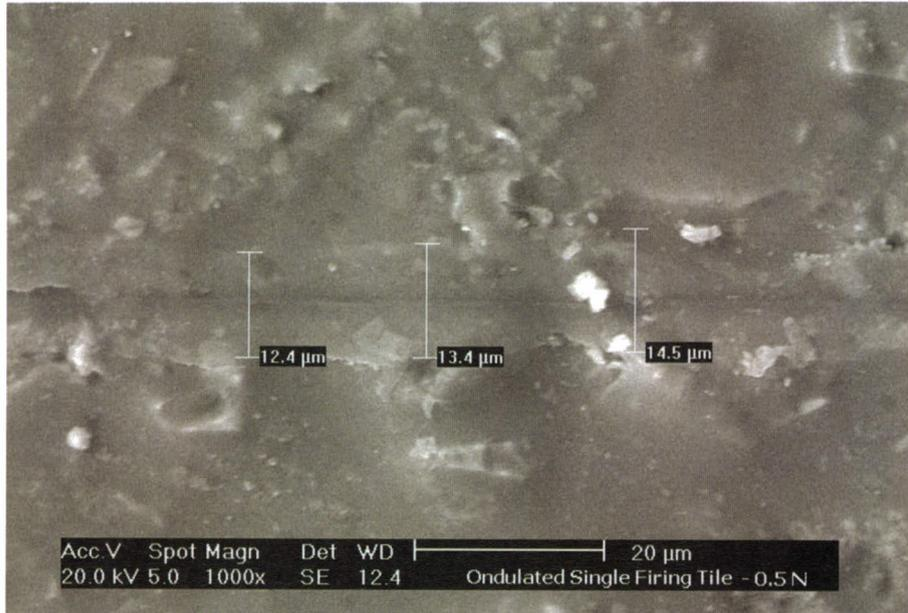
Figure 7. Scratch in the second type of single-fired wall tile
