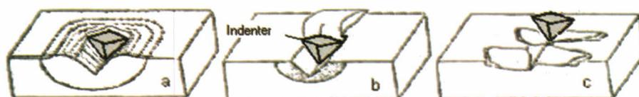
Figure 1. Material loss mechanism
