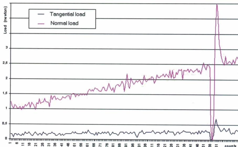
Figure 11. Identification of the critical load for scratch transition of the glass-ceramic tile
