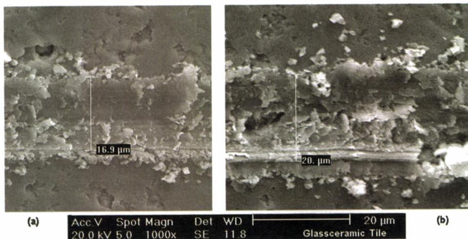
Figure 9. Scratch in the glass-ceramic tile using: (a) 0.5 N and (b) 1.0 N
