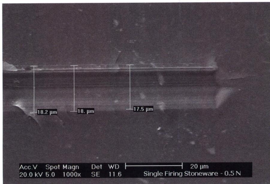
Figure 6. Scratch in the first type of single-fired tile
