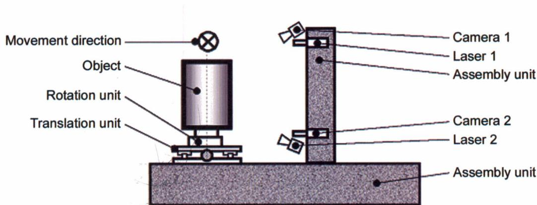
Figure 10. Schematic illustration of the 3D digitizer.
