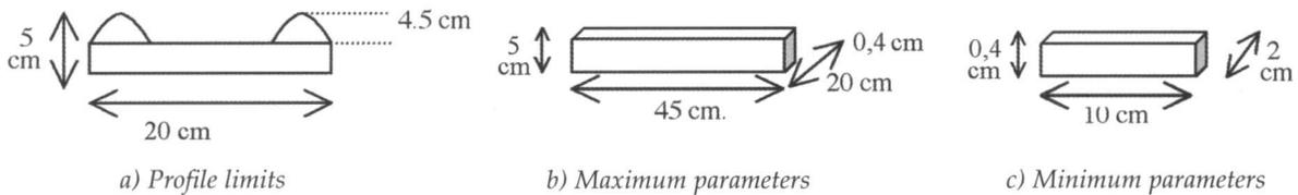
Figure 5. Graphic illustration of the profile of a border and its limits.
