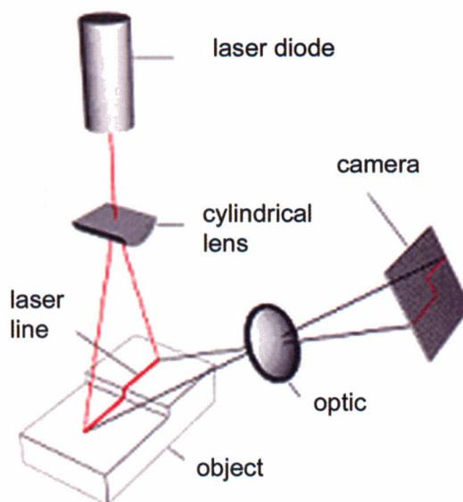
Figure 11. Principle of the laser sensors used.
