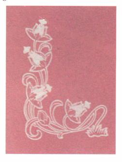
Figure 5. Decoration of the engobe layer. The depth effect is more pronounced with increasing glaze layer thickness. Design resolution: 1270 dots/inch.
