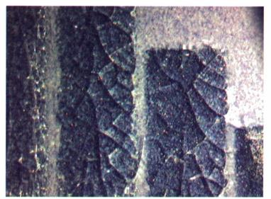
Figure 2. Glaze crazing produced by the laser beam.
