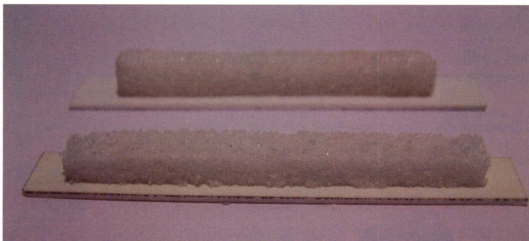
Figure 3. Sample of incoherent granular frit before (in the foreground) and after the thermal expansion and sintering test.
