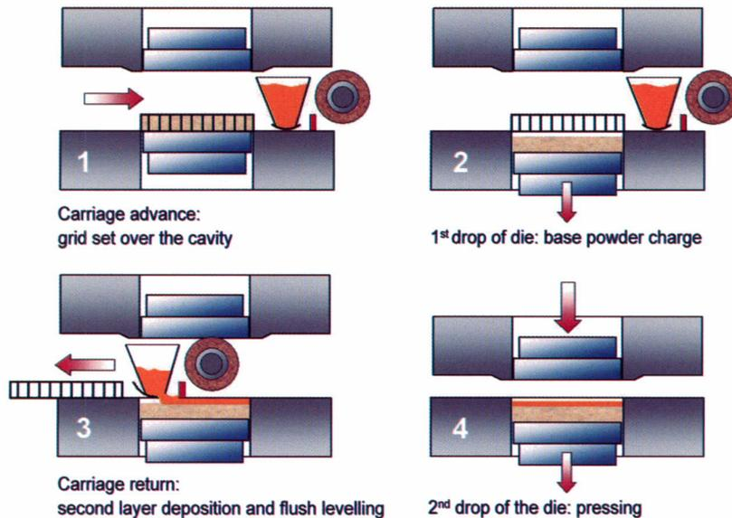
Figure 2. Schematic of the double-charge operation
