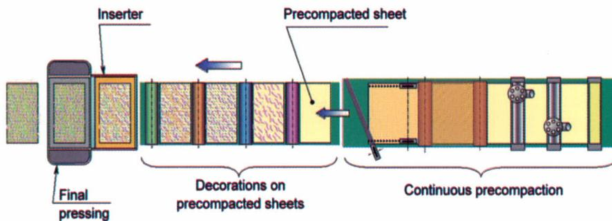
Figure 12. Schematic of a continuous precompaction line
