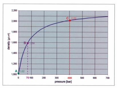
Figure 6. Compaction characteristics of a porcelain tile body
