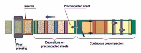
Figure 12. Schematic of a continuous precompaction line
