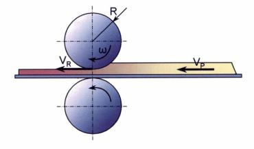
Figure 5. Conceptual scheme of continuous precompaction
