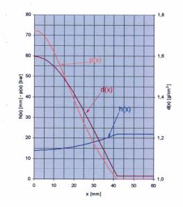
*Figure 8. Variation of* h(x)*,* d(x) *and* p(x) *(cylindrical roller)*
