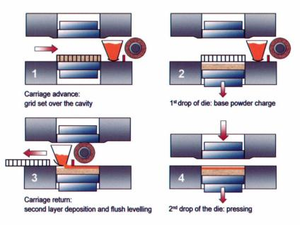
Figure 2. Schematic of the double-charge operation
