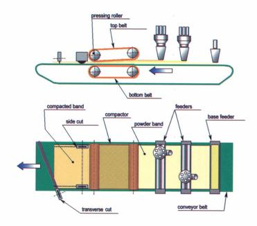
Figure 10. Schematic of continuous precompaction
