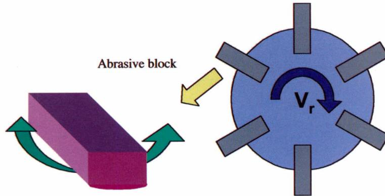
Figure 1. Schematic diagram of typical swinging head grinding tool used in industrial polishing process.
