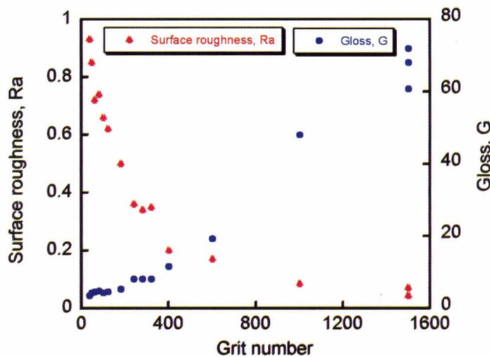
Figure 9. Surface roughness Ra and gloss G as a function of grit number of abrasive pin for the full sequence of polishing steps in the laboratory test.
