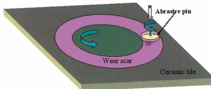
Figure 8 Sample and abrasive pin motion used in the laboratory tests
