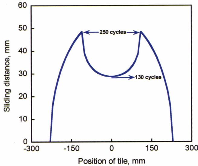
Figure 4 The number of contact cycles and sliding distance of a ceramic tile as a function of position of the material with respect to the centre-line of the tile (axis of rotation of the abrasive).
