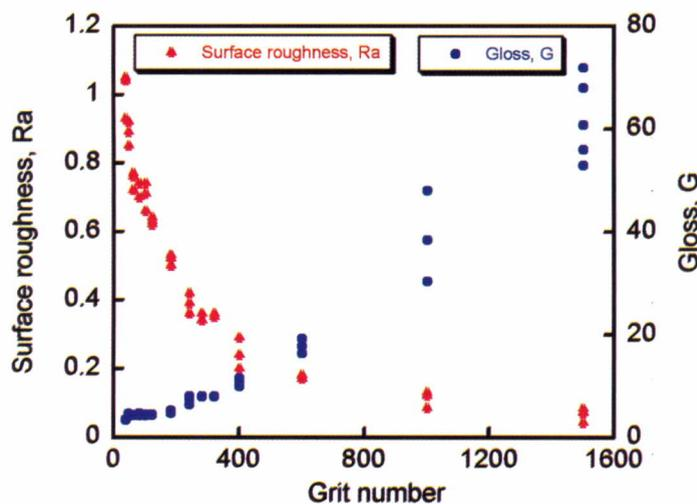
Figure 10. Surface roughness Ra and gloss G of the polished tile surface after 60 seconds exposure to each abrasive pin. In the case of 1500 grit, the three data points relate to 60, 180 and 300 seconds exposure.
