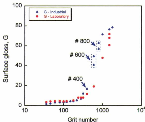
Figure 11 Comparison of gloss values for samples from the industrial polishing line and the laboratory tribometer.
