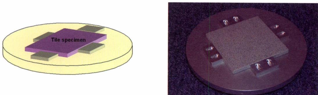
Figure 6 (a) Schematic diagram of ceramic tile specimen holder; (b) Actual part.
