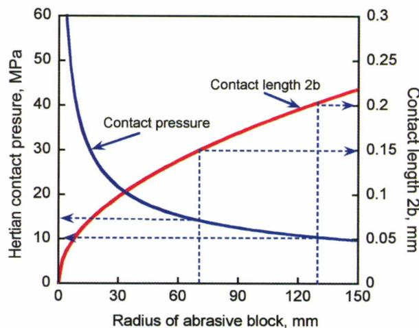
Figure 3. Change in contact pressure and contact length during the polishing process as a function of the radius of curvature of the abrasive block.
