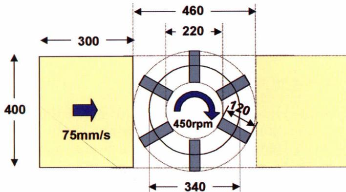
Figura 2. (a) Schematic diagram showing the dimensions of the grinding tool in the polishing process;
