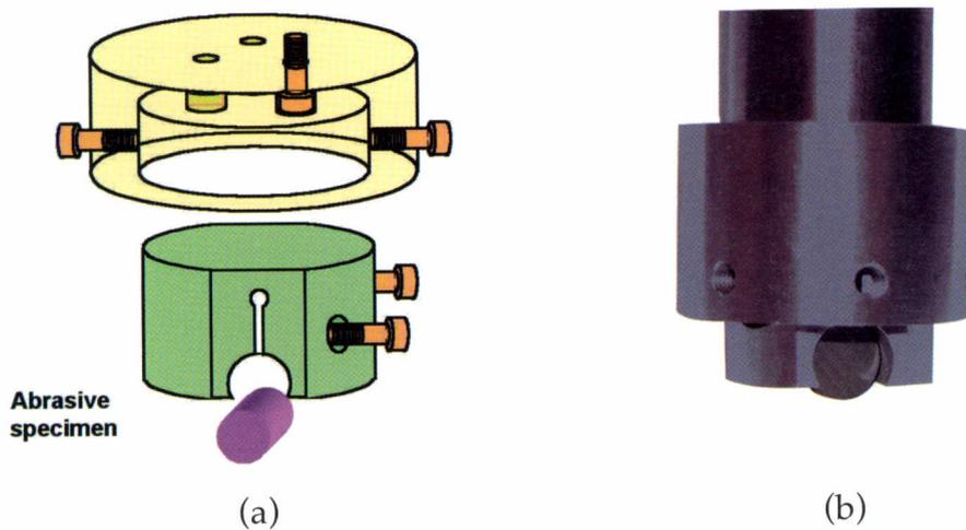
Figure 7 (a) Schematic diagram of abrasive pin, holder and coupling; (b) Assembly of abrasive pin, holder and coupling.
