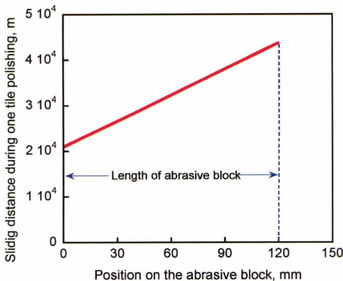
Figure 5 Sliding distance on abrasive block as a function of distance from the end of the block.
