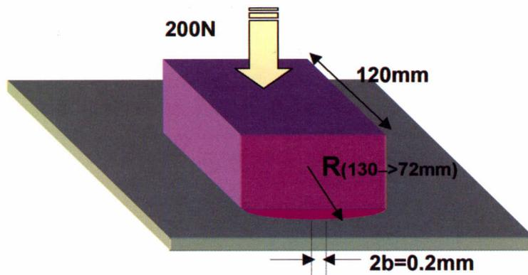
Figura (b) Relative motion between abrasive block and ceramic tile in the polishing process.
