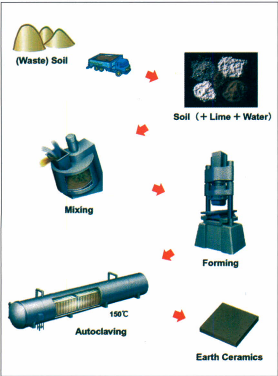
Figure 14. Actual Processing of Earth Ceramics Manufacturing.
