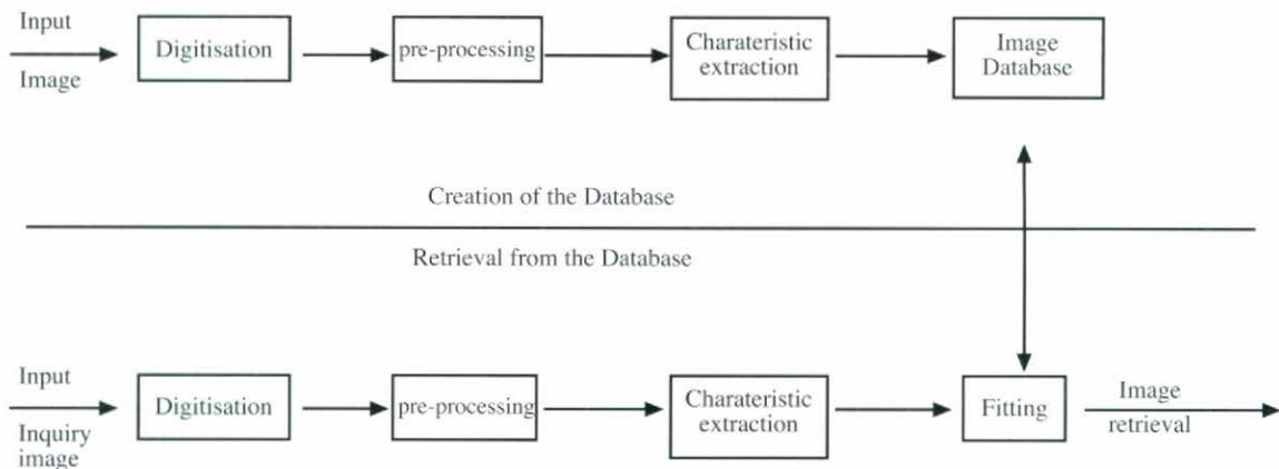
Fig. 2.1 Structure of the system.
