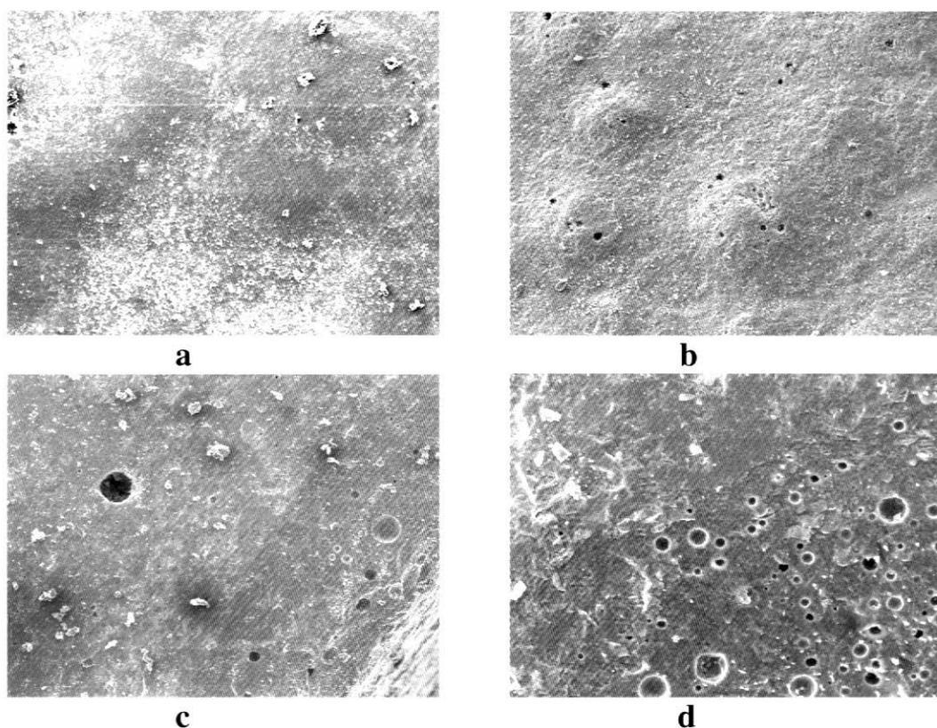
Fig. 3. Image of the surface of glazed tiles after testing their abrasion resistance (2100 abrasion cycles):
