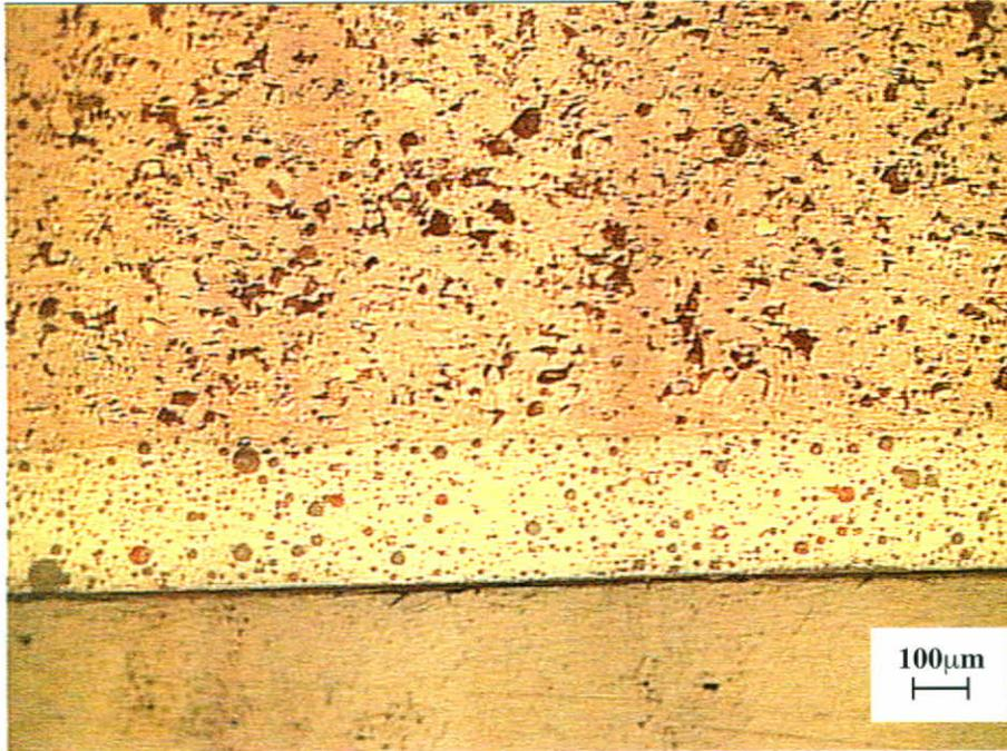
Fig. 3. Optical Micrograph displaying the general aspects of glaze/body interface in a vitrified stoneware floor tile mass fast fired at 1150°C during 3 minutes in a conventional electric furnace. Heating/cooling rate used was 50°C/minute.
