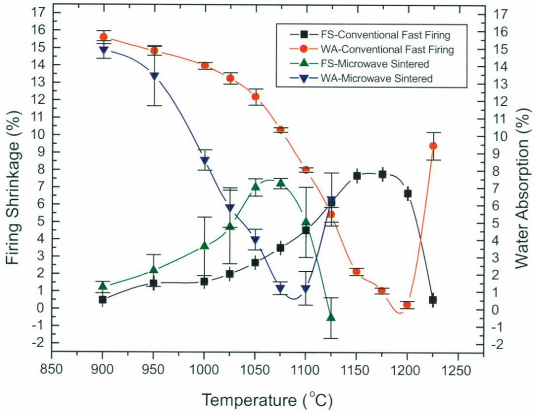
Fig. 1. Vitrification Diagrams for the Conventionally and Microwave fired specimens of vitrified floor tile composition.
