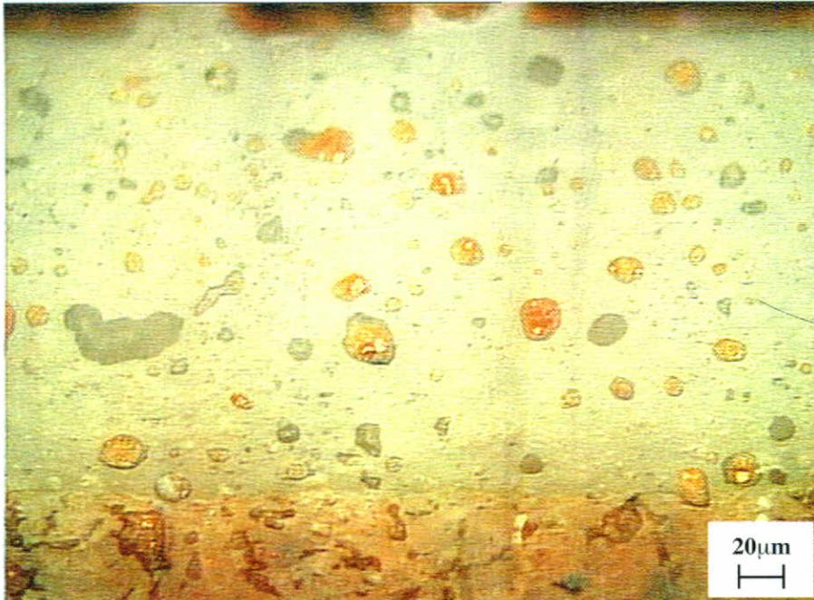
Fig. 4. Optical Micrograph showing the general aspects of glaze/body interface and glaze bulk, of a single fired glazed vitrified stoneware floor tile mass under microwave energy at 1050°C for 3 minutes under 50°C/minute heating rate.
