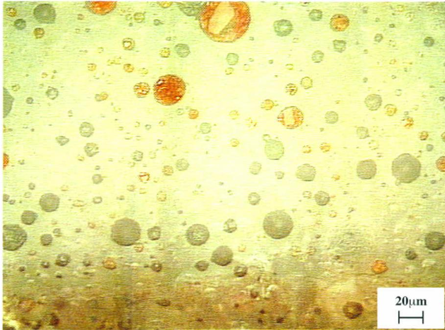
*Fig. 5. Optical Micrograph showing the general aspects of glaze/body interface and glaze bulk, of a single fired in a conventional vitrified glazed stoneware floor tile mass in conventional electric furnace during 3 minutes under heating/cooling rate of 50°C/minute.*
