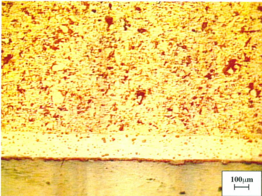
Fig. 2. Optical Micrograph displaying the general aspects of glaze/body interface in a vitrified stoneware floor tile mass single fired under microwave energy at 1050°C during 3 minutes. Heating rate 50°C/minute.
