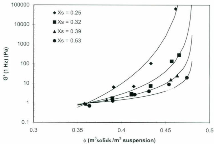
Figure 3. Relation between  $G'$  and  $\phi$ . Verification of the proposed model.
