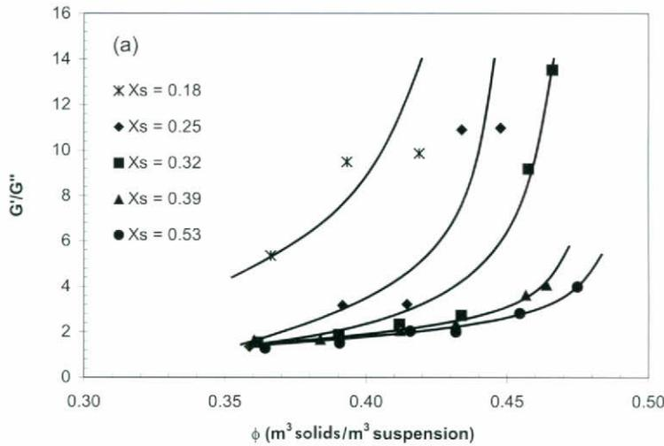
Figure 2. Effect of solids volume fraction,  $\phi$ , and deflocculant content,  $X_s$ , on the ratio  $G'/G''$ .
