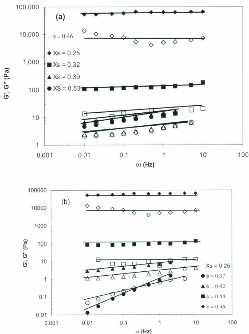
Figure 1. Variation of  $G'$  and  $G''$  with oscillation frequency,  $\omega$ . (a) Experiments at  $\phi=0.46$ . (b) Experiments at  $X_s=0.25$ . ( $G'$  solid symbols,  $G''$  empty symbols).
