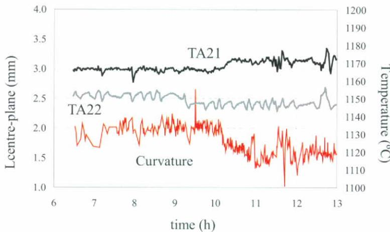
Figure 1. Reduction in tile curvature caused by changes in the set top thermocouple temperature TA21.
