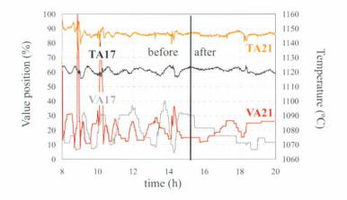
Figure 3. Modification of valve control parameters.
