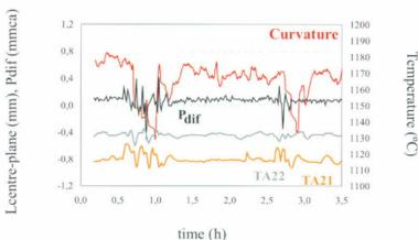
Figure 2. Effect of gaps on tile curvature.
