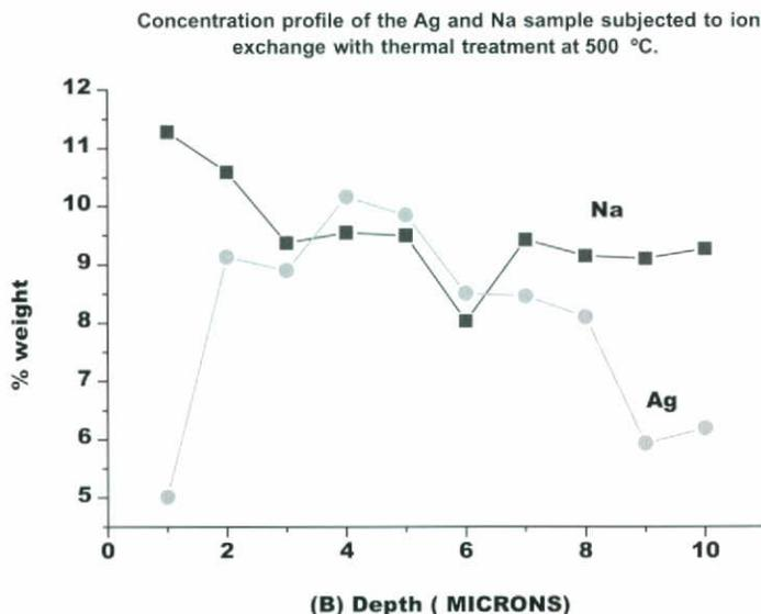
Figure 3. Sodium and silver concentration profile in a glass sample, with and without thermal treatment (B and A, respectively).
