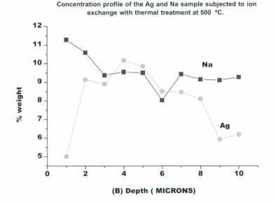
Figure 3. Sodium and silver concentration profile in a glass sample, with and without thermal treatment (B and A, respectively).
