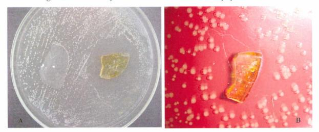
Figure 4 - Samples of ionic exchanged glasses. A) Inhibition halo with Staphylococcus aureus. B) Inhibition halo with Escherichia coli.
