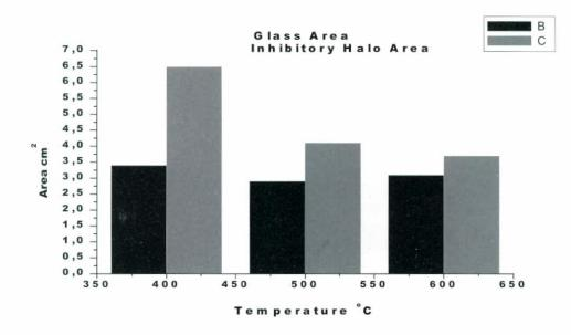
Figure 2. Effect of glass thermal treatments on microbial growth.
