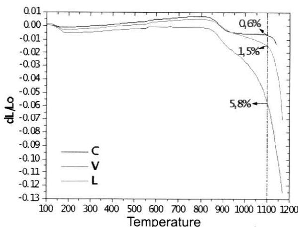
Figure 1 – Plots of thermal dilatometric analysis corresponding to clays C, V and L.
