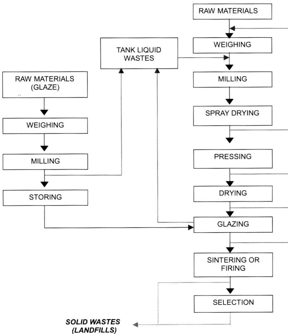
Figure 1. Flowchart of the ceramic floor tile production process.
