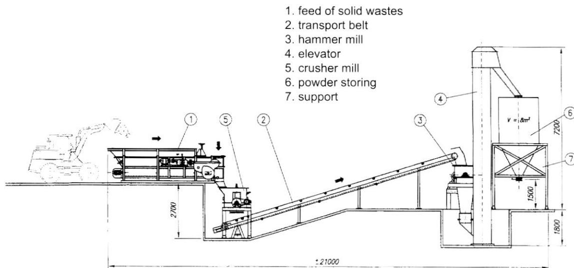
Figure 2. Recycling plant lay out.
