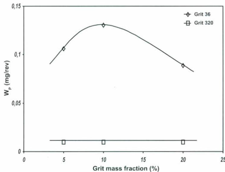
Figure 6. Effect of grit mass fraction on porcelain tile wear rate.
