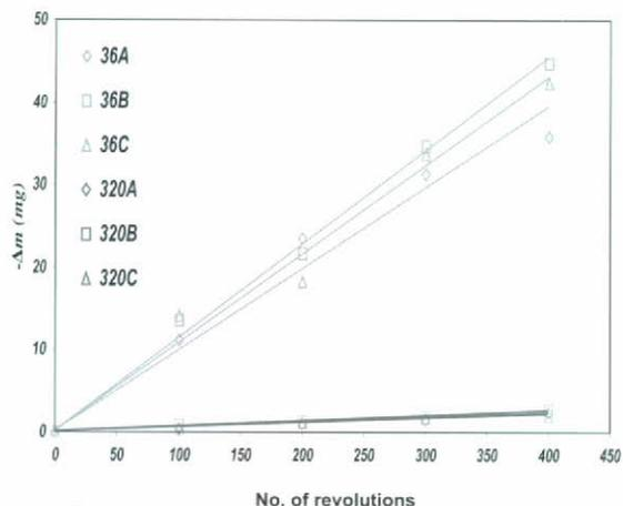
Figure 12. Grinding tool behaviour during the wear test.
