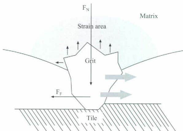
Figure 13. Scheme of abrasive grain action on the cement matrix.
