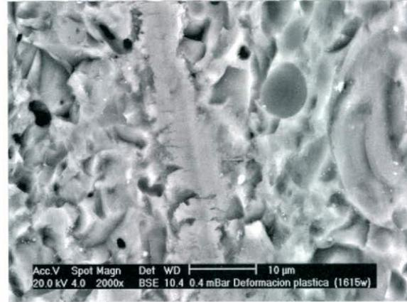
Figure 11. Scratching mechanism by plastic strain.
