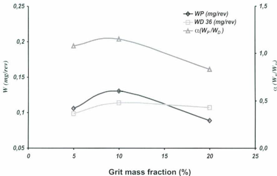
Figure 15. Effect of grit size on grinding tool efficiency.
