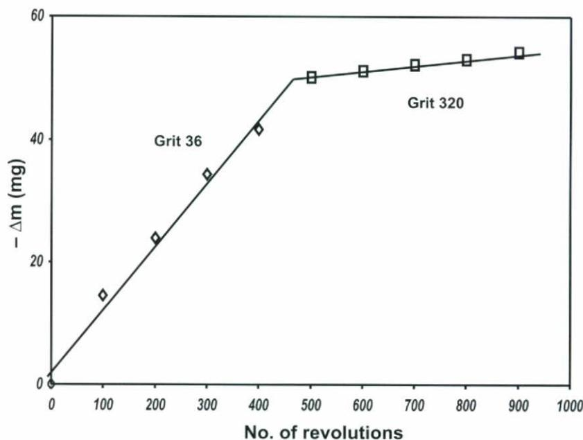
Figure 16. Change of wear rate produced by the different grit sizes used.
