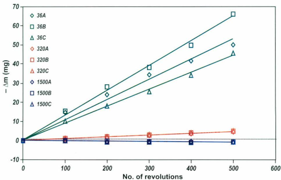
Figure 5. Porcelain tile specimen behaviour during the wear test.
