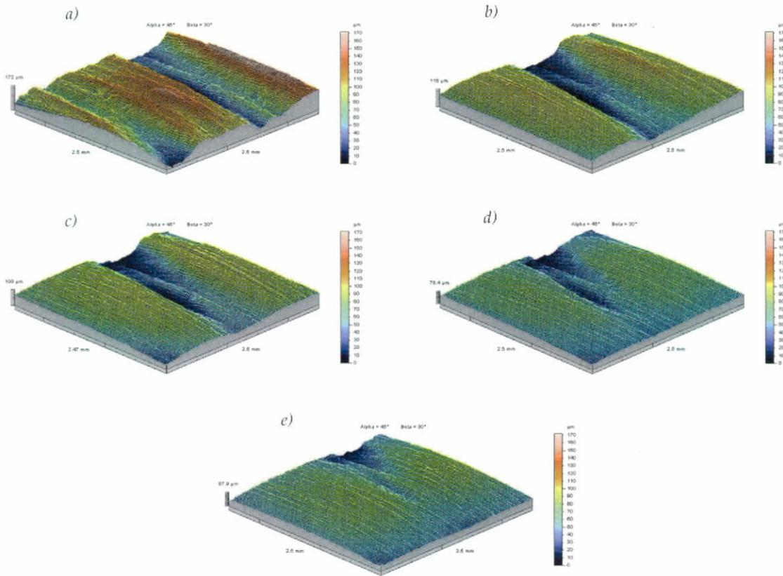
Figure 17. Topographic map of the abraded porcelain tile test specimen surface: a) with grit 36; b) after 100 revolutions with grit 320; c) after 200 revolutions with grit 320; d) after 300 revolutions with grit 320; and e) after 400 revolutions with grit 320.
