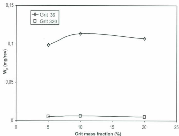
Figure 14. Variation of abrasive disk wear rate versus grit mass fraction in the disk.
