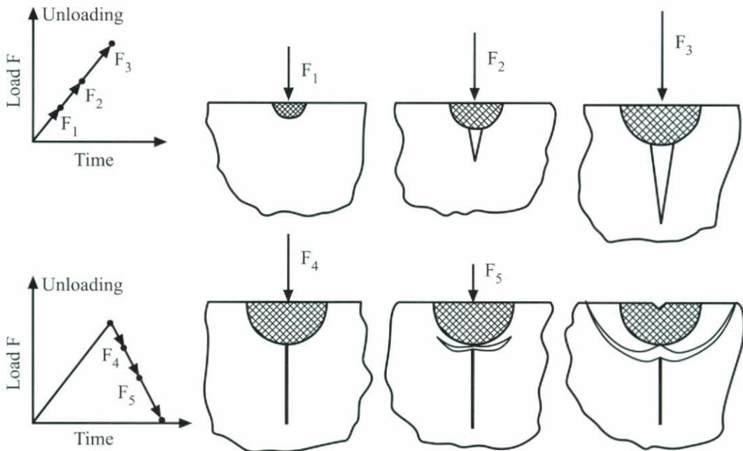
Figure 9. Scratch generation mechanism by static indentation (Source: ref. [6]).
