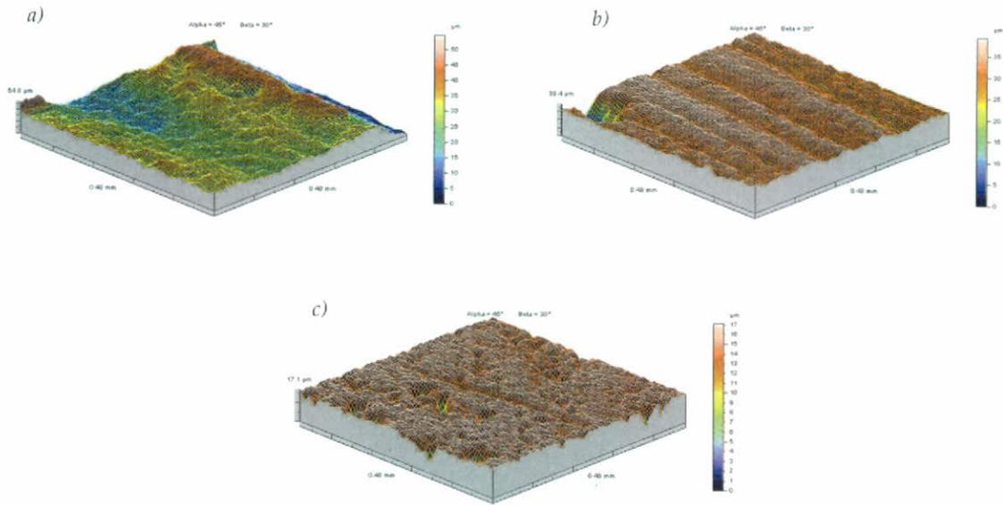
Figure 8. Topographic maps (0.48x0.48 mm) of test specimen surfaces abraded with discs containing variously sized grit: a) grit 36; b) grit 320; c) grit 1500.
