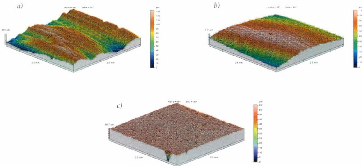
Figure 7. Topographic maps (2.5x2.5 mm) of the test specimen surfaces abraded with disks containing different grit sizes: a) grit 36; b) grit 320; c) grit 1500.
