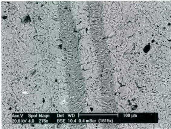
Figure 10. Scratches produced by 320 grit.
