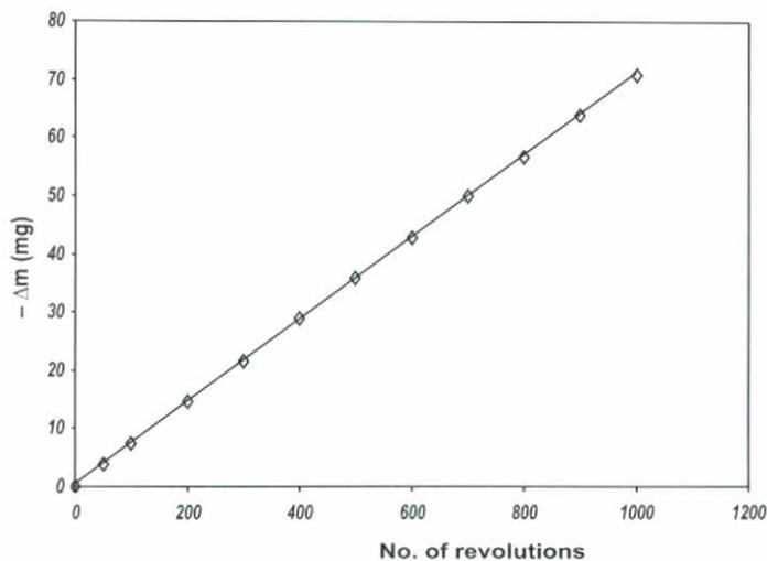
Figure 2. Wear test with a wedge-shaped pin.
