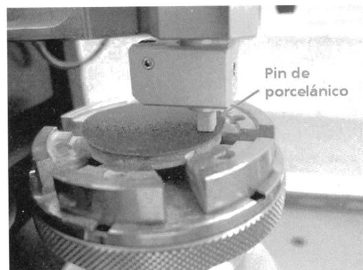
Figure 1. Pin-on-disk arrangement in the tribometer.
