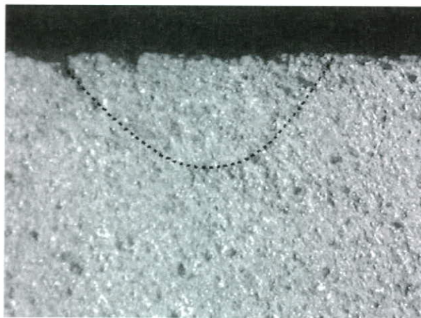
Figure 6. Pseudo-plastic fracture in a stoneware body.
