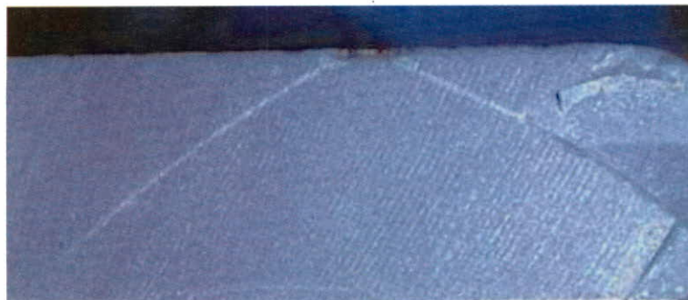
Figure 5. Hertzian fracture in a porcelain tile.
