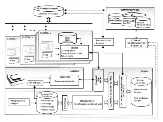
Figure 5. Collaborative environment architecture for redesign tasks in the ceramic and textile industry.
