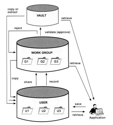
Figure 3. Generic structure of a PDM system.
