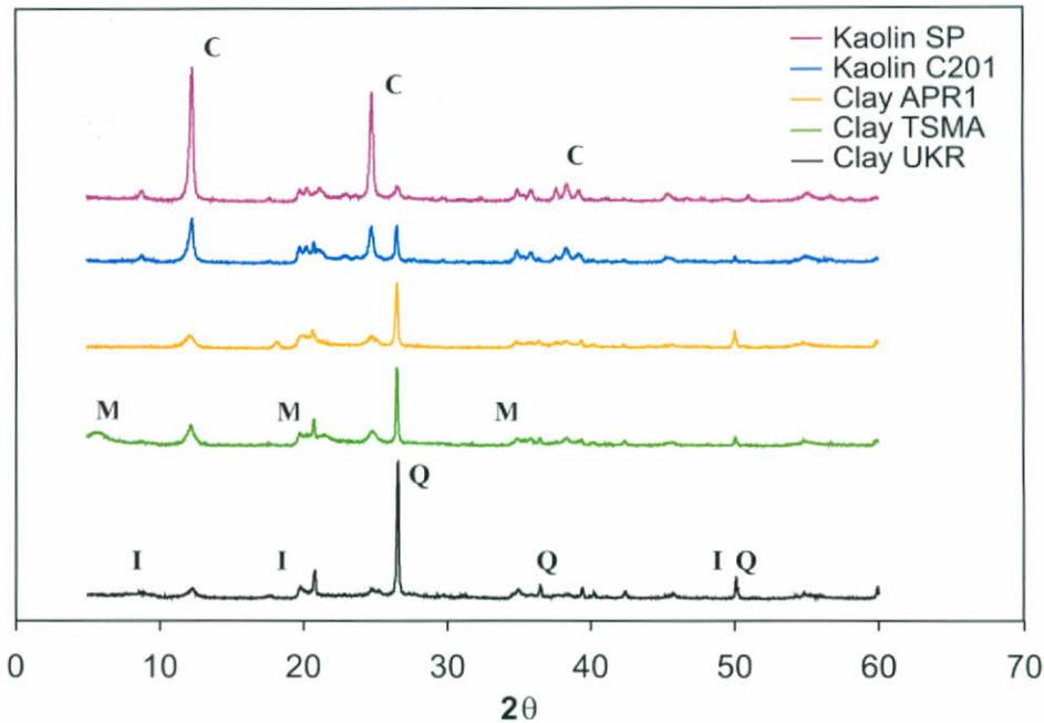
Figure I: Diffractograms of the studied clays: C(Kaolinite), M(Montmorillonite), I(Illite), Q(Quartz).
