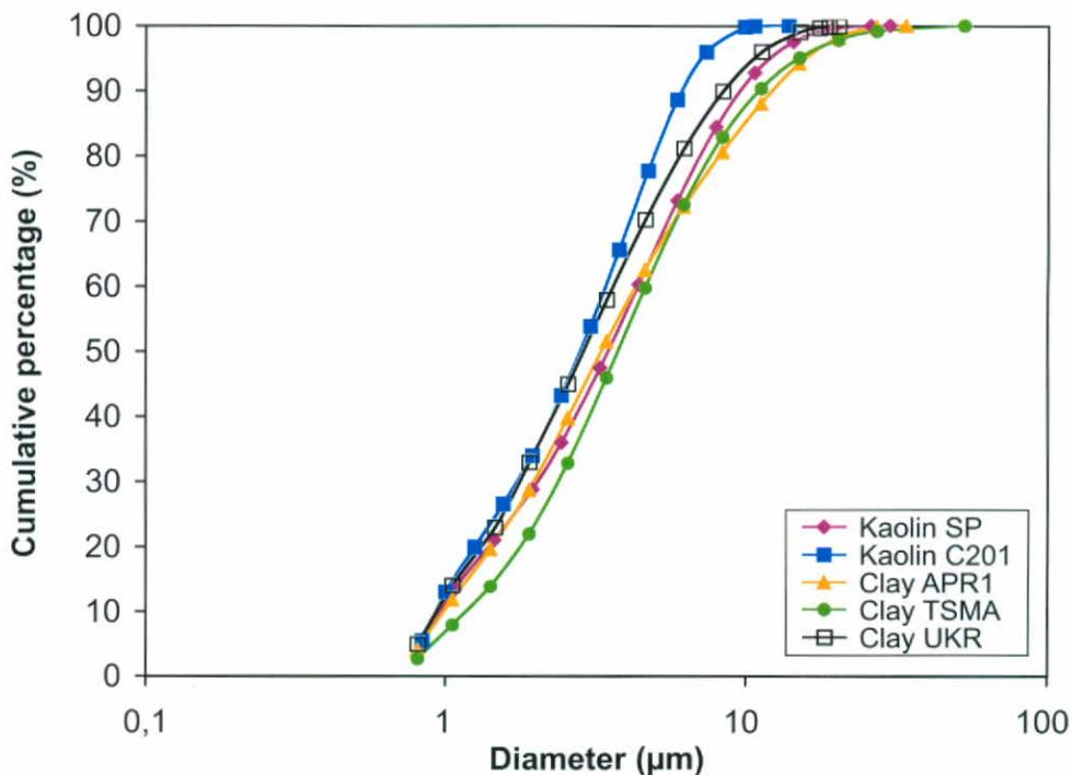
Figure II: Cumulative particle size distribution of the clays.
