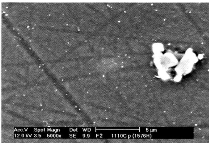
Figure 15. Microstructure of a specimen of frit F2 + 1% pigment produced with standard cooling .
