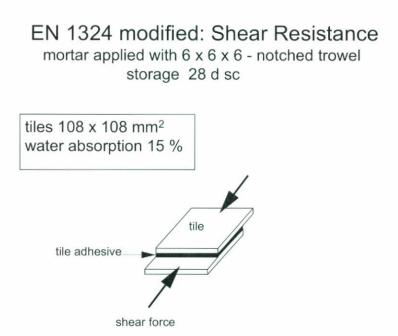
Figure 7: specimen acc. to EN 1324.
