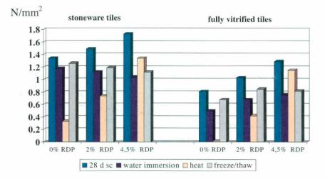
Figure 3: tensile adhesive strength correlated with type of tiles and amount of polymer used.
