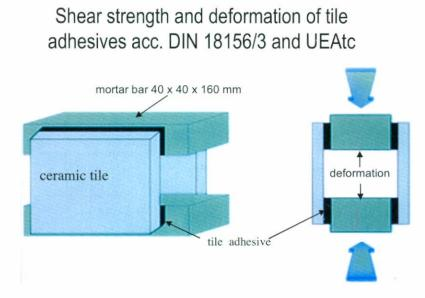
Figure 4: shear test acc. to UEAtc / DIN 18156/3, scheme of test configuration.
