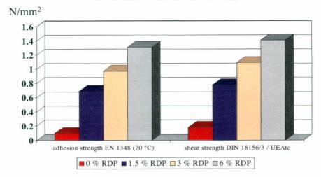
Figure 6: shear resistance acc. to DIN 18156/3 compared with the tensile adhesive strength acc. to EN 1348.
