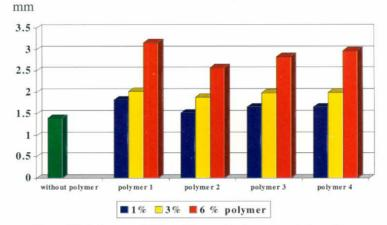
Figure 10: influence of different types of polymers on deformation.
