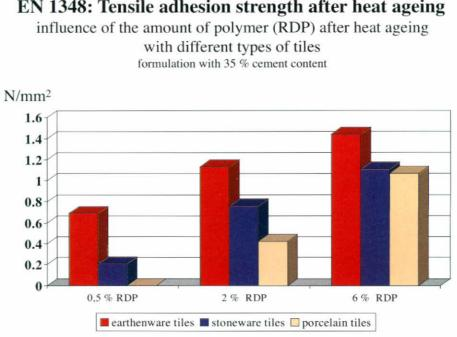
EN 1348: Tensile adhesion strength after heat ageing
