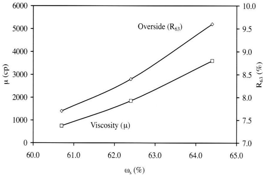
Figure 2. Variation of viscosity and oversize with solids content (laboratory tests).
