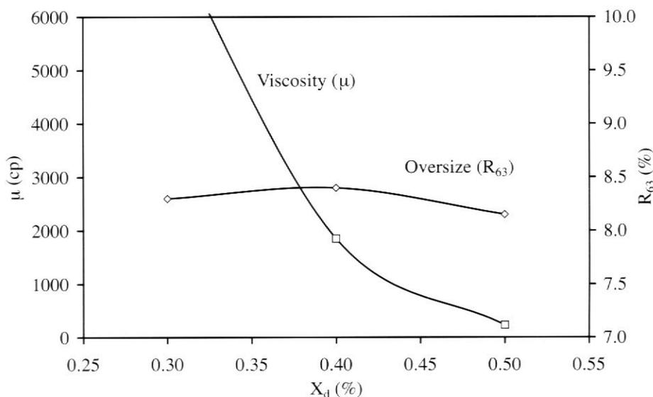
Figure 4. Variation of viscosity and oversize with deflocculant content (laboratory tests).
