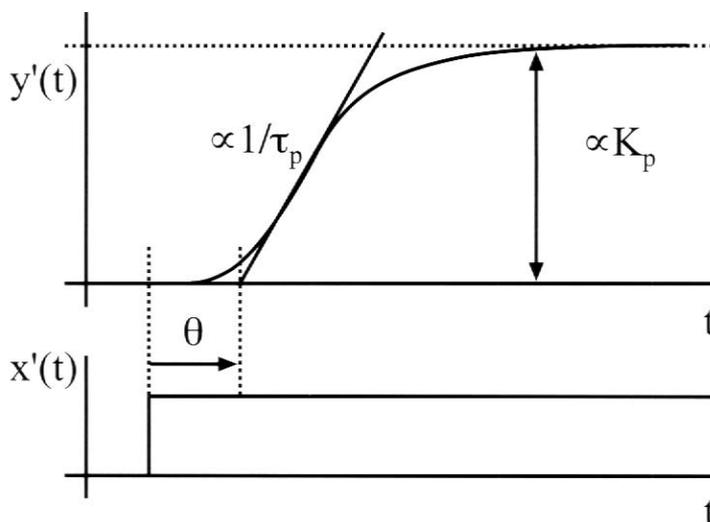
Figure 5. Physical meaning of the parameters involved in the dynamic model.
