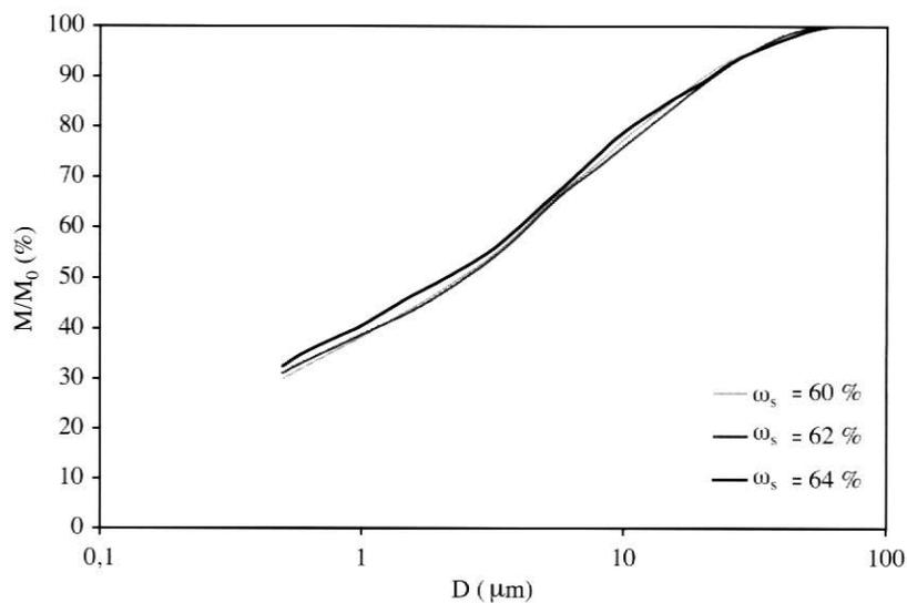
Figure 3. Variation of particle size distribution with solids content (laboratory tests).
