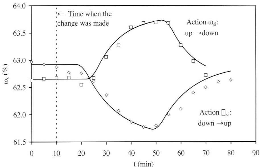
Figure 6. Theoretical fit of solids content at the mill exit.
