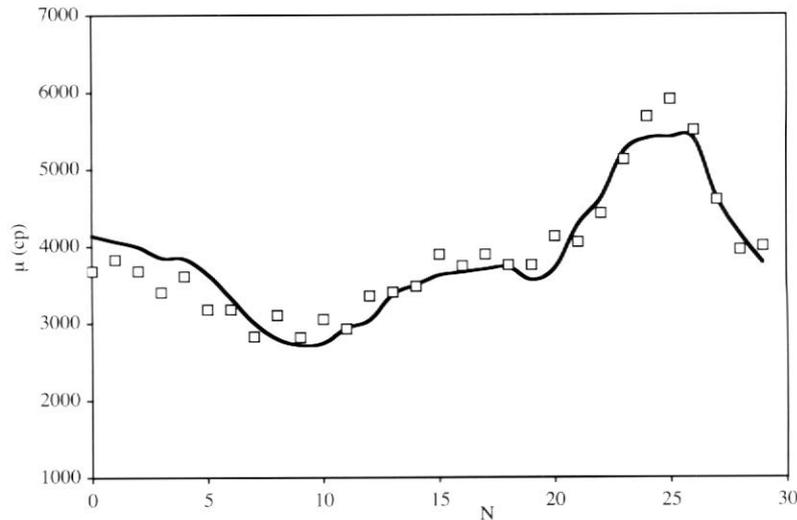
Figure 10. Theoretical fit of viscosity with the Krieger- Dougherty equation.
