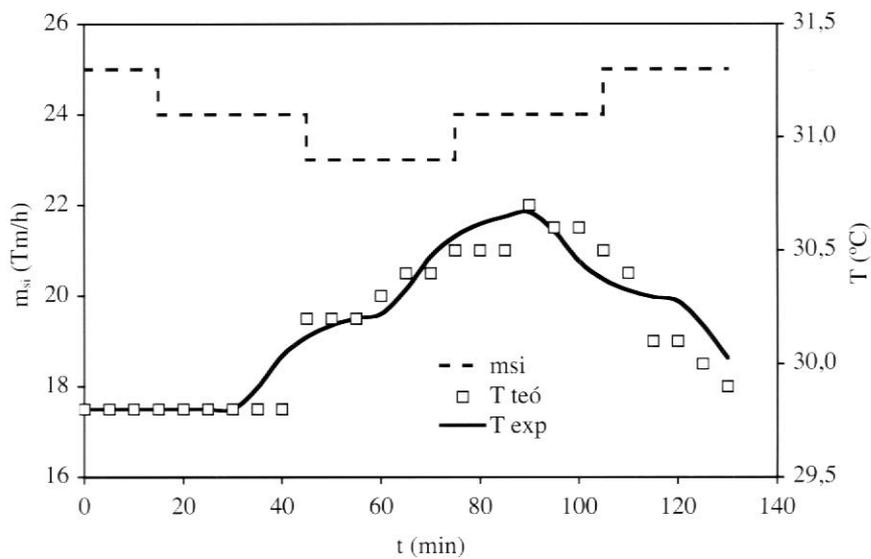
Figure 15. Effect of solids feed flow rate on suspension temperature.
