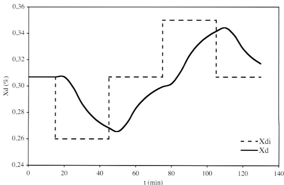
Figure 14. Estimated elapsing time between mill input deflocculant content ( $X_{di}$ ) and mill output deflocculant content ( $X_d$ ).
