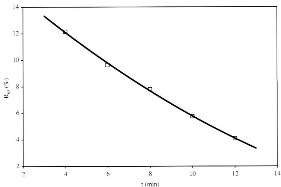
Figure 1. Relation between milling time and mass oversize at 63  $\mu\text{m}$  (laboratory test).
