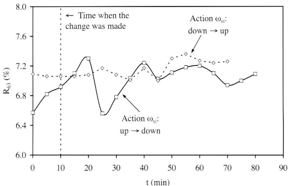
Figure 7. Plot of oversize on raising input solids content.
