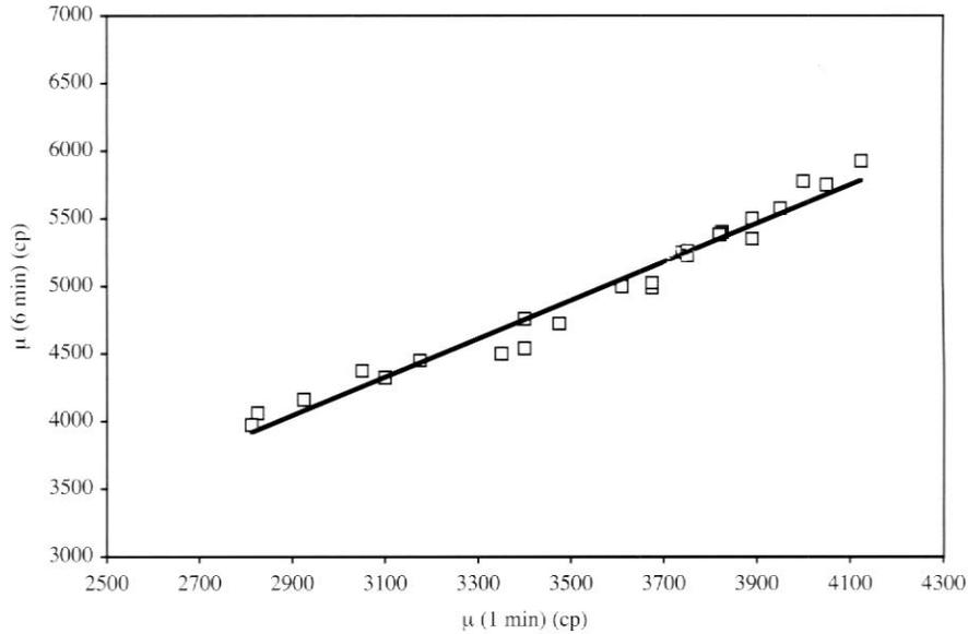
Figure 9. Relation between measured viscosity after 1 and 6 min suspension rest on modifying solids content.
