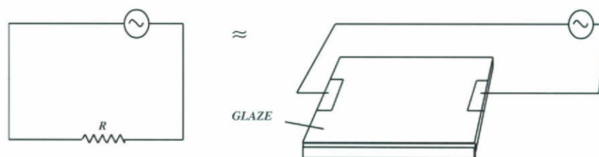
Fig. 11. Scheme of the ceramic tile set in a resistive circuit in AC.
