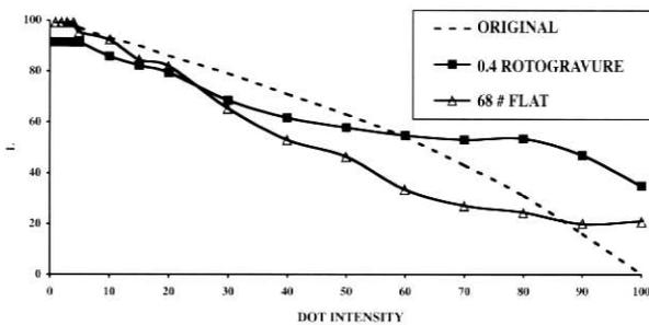
Fig. 25: Comparison of black and matt ink colorimetries. 0.4 rotogravure print – 68 # flat screen.
