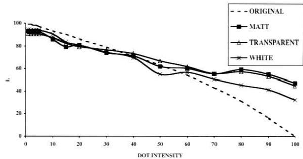
Fig. 30: Comparison of black ink colorimetries on different glazes. Rotogravure roller. 0.3 definition.
