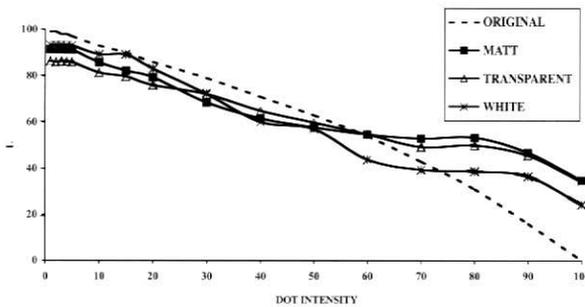
Fig. 29: Comparison of black ink colorimetries on different glazes. Rotogravure roller. 0.4 definition.
