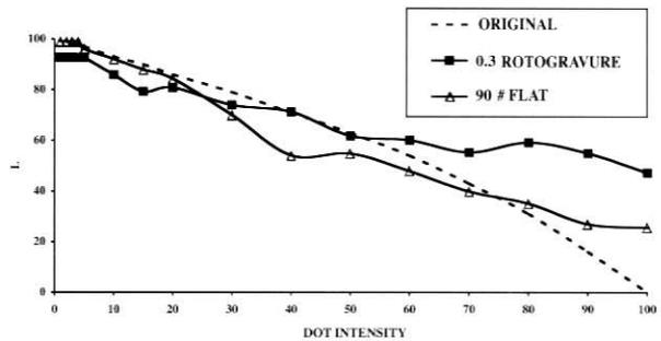
Fig. 26: Comparison of black and matt ink colorimetries. 0.3 rotogravure print – 90 # flat screen.
