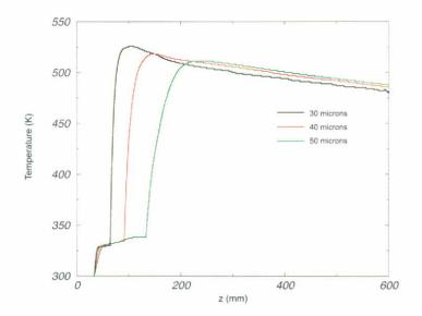
Figure 5: Droplet temperature along their trajectories inside the drying chamber.
