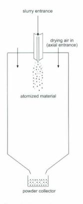
Figure 2: Spray drying chamber of concurrent flow.
