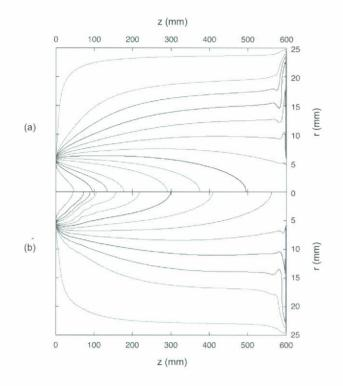
Figure 6: Air isotherms (a) before and (b) after the droplet injection. Inner line of 580 K, decreasing in intervals of 10 K.
