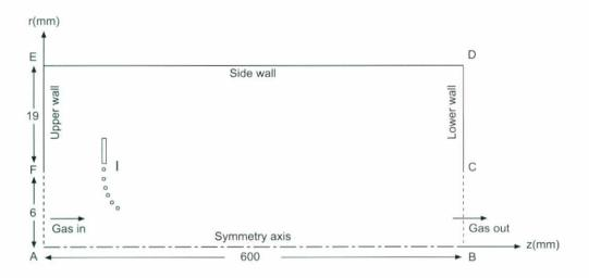
Figure 1: Computational domain of a spray drying chamber.
