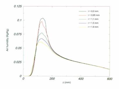
Figure 9: Air humidity after the droplet injection. Axial profiles ( $0 \le z \le 5$  mm).
