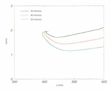
Figure 4: Droplet trajectories inside the drying chamber. Mixed flow with injection angle of 270° (nozzle tip parallel to the chamber axis).
