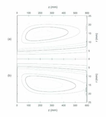
Figure 7: Air stream lines (a) before and (b) after the droplet injection. Inner line (the nearest to the symmetry axis) of 0.001 g/s, increasing in intervals of  $2 \times 10^{-2}$  g/s.
