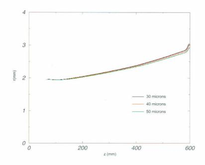
Figure 3: Droplet trajectories inside the drying chamber. Concurrent flow with injection angle of 90° (nozzle tip parallel to the chamber axis).
