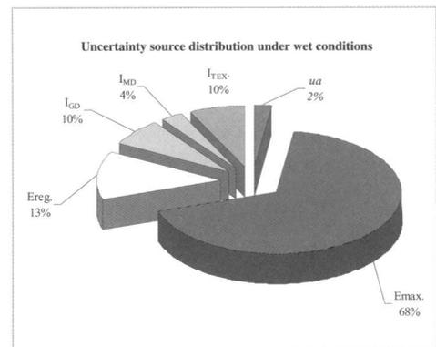
Figure 13. Distribution of the uncertainty sources of the measurement process with the Tortus system under wet conditions and a smooth surface.
