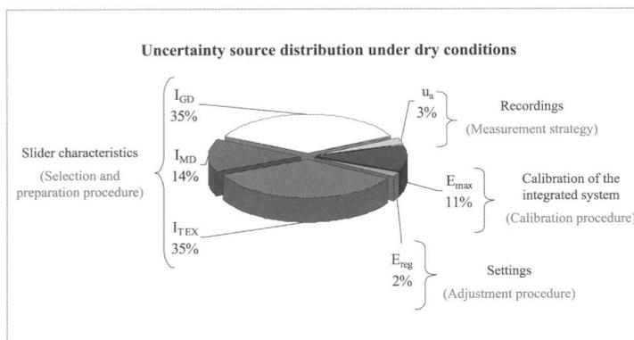
Figure 12. Uncertainty source proportions in the measurement process with the Tortus system under dry conditions and a smooth surface.
