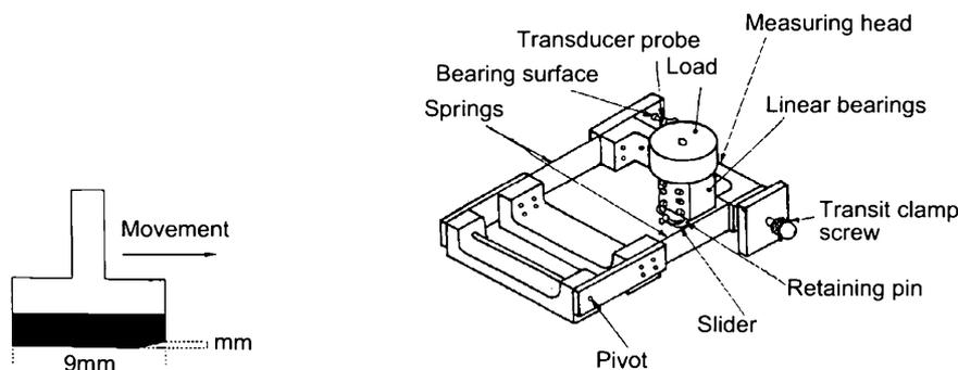
Figure 2. Shape of the rubber slider.
