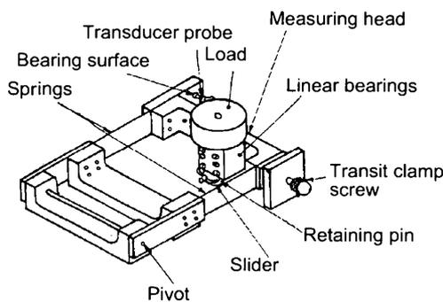
Figure 3. Tortus measurement system: force transducer.
