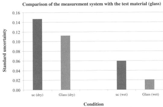
Figure 10. Results of the uncertainty of the measurement system and variable to be measured (glass).
