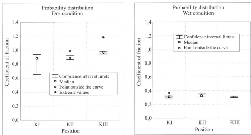
Figure 8. Variation of the coefficient of friction on the reference plate under wet and dry conditions.
