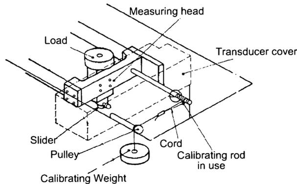
Figure 4. Adjustment of Tortus system gain.
