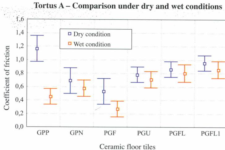
Figure 14. Results of the coefficient of friction on ceramic floor tiles.
