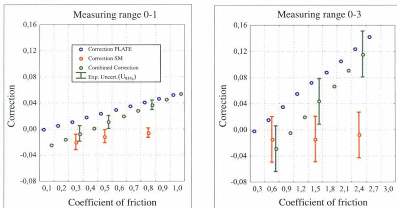
Figure 6. Curve resulting from the calibration of Tortus A.
