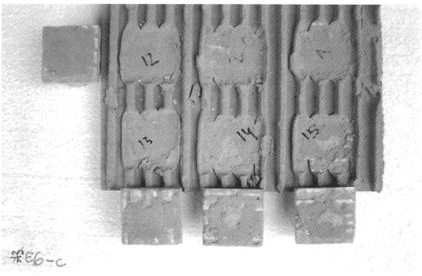
*a5. Detail of a bonding test specimen.*
