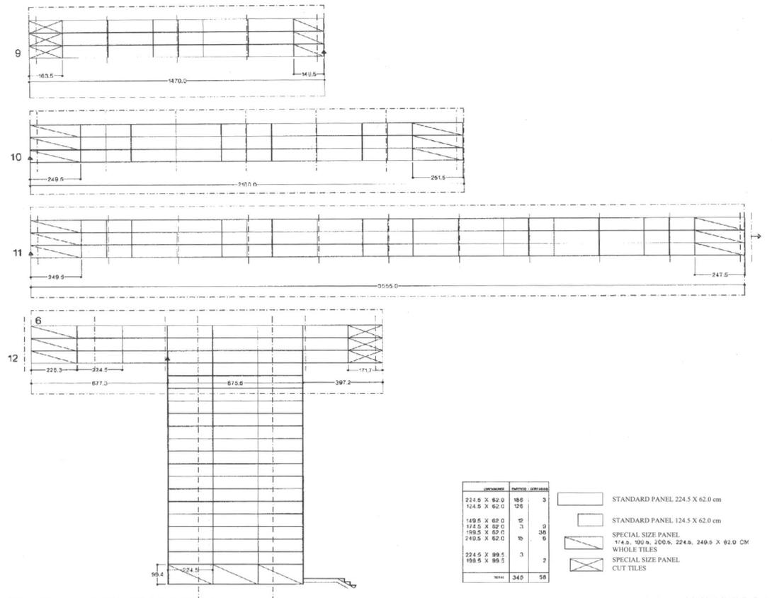
Figure 2. Panel set out drawing in part of the roof and stairs.
