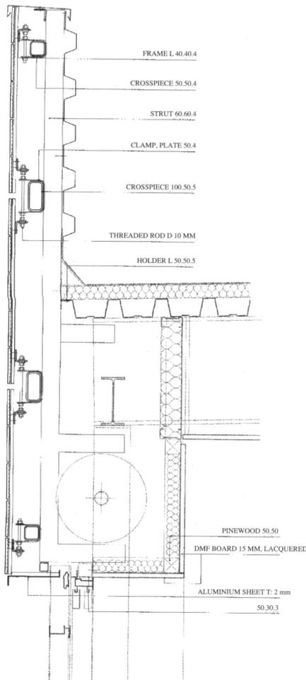
Figure 1. Standard cross section of the roof parapet.
