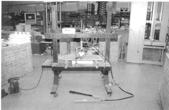
*a1. Complete bending strength test configuration.*
