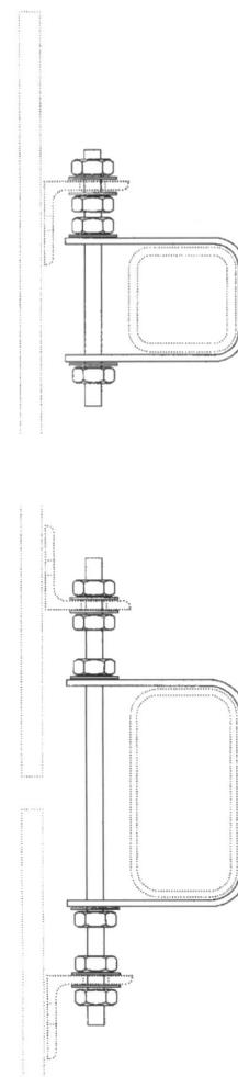
*Figure 4. Underlying frame anchorings to the panel.*
