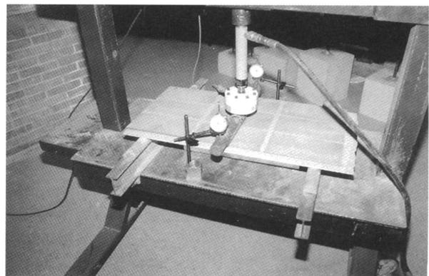
*a2. Bending strength test. Detail.*
