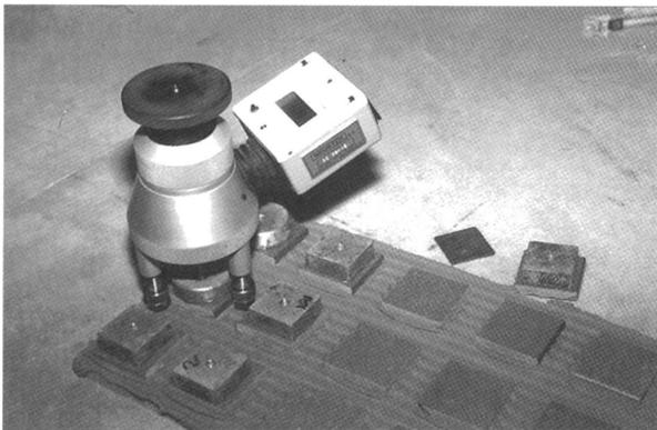
*a3. Bonding tests. Tile pull configuration.*
