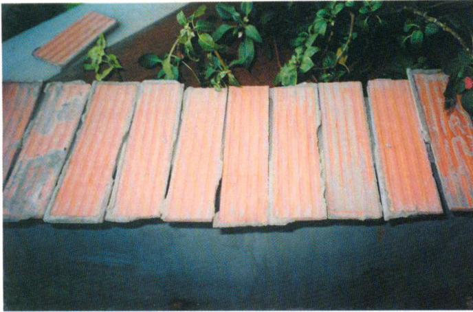
*Figure 3. Tiles removed from the facade show problem of fixing. Inadequacy of setting together with wrong specification of material caused failure.*
