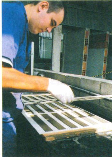
**Figure 21.** The apparatus shown was designed and built to make the flexibility test easier and cheap. Goods results showed its applicability. The apparatus costs about US\$ 1,000.
