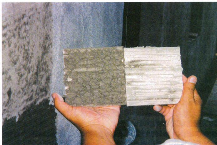
*Figure 7. Left: full coverage where accurate setting was used. Right: the lack of adhesive material often causes failure. Technique, tools and quality control play an important role.*
