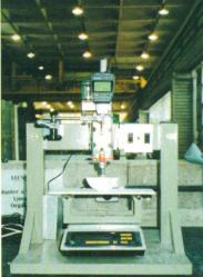
Figure 21. The apparatus shown was designed and built to make the flexibility test easier and cheap. Goods results showed its applicability. The apparatus costs about US\$ 1,000.
