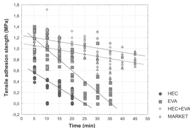
**Figure 5.** Open time linear regression for the studied mortars.
