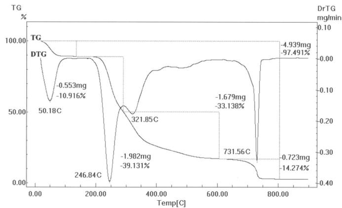
Figure 4. HEC thermogravimetry result (TG)
