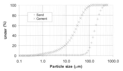
Figure 1. Laser granulometry of Portland cement and sand.
