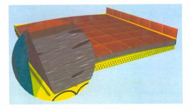
This problem occurs especially in fast drying floors. In slow drying, as mentioned above, there is a clear drop in the shrinkage coefficient and in deformation behaviour. It is furthermore to be noted that floor quality is heightened by slow drying, with regard to compression resistance and bending tensile strength. Slow drying is achieved in particular by good curing.
