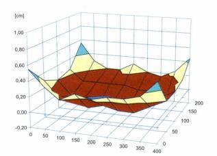
Cement mortar screed without ceramic tiles. Measurement after 28 days).
