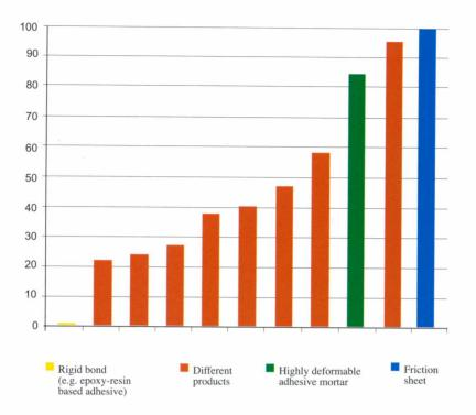
Not all adhesive mortars are sufficiently deformable. The stress absorption capability of various adhesive mortars was determined at PCI Augsburg, monitoring surface stresses.
