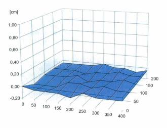
Cement mortar floor covered with ceramic tiles after 2 days. Measurement after 28 days.
