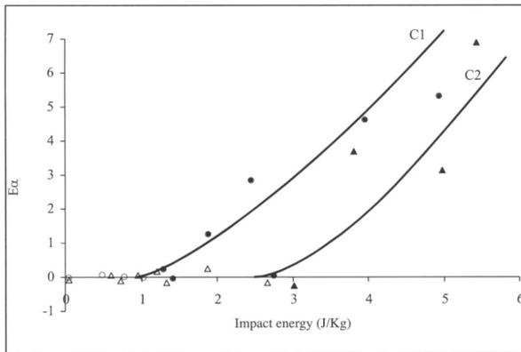
Figure 3. Impact test results of tiles C1 and C2.
