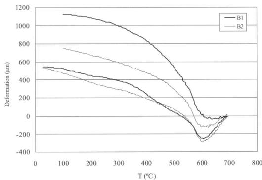
Figure 5. Glaze-body fit of tiles B1 and B2.
