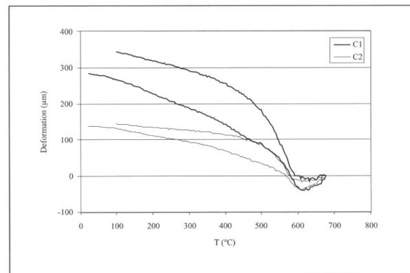
Figure 6. Glaze-body fit of tiles C1 and C2.
