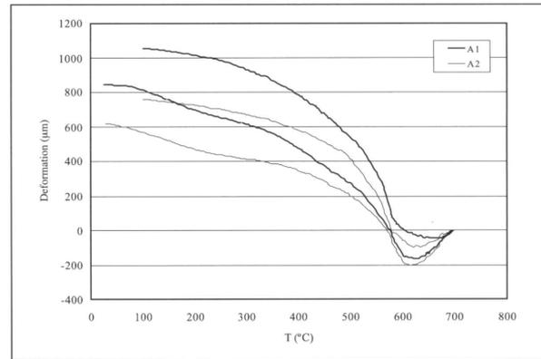
Figure 4. Glaze-body fit of tiles A1 and A2.
