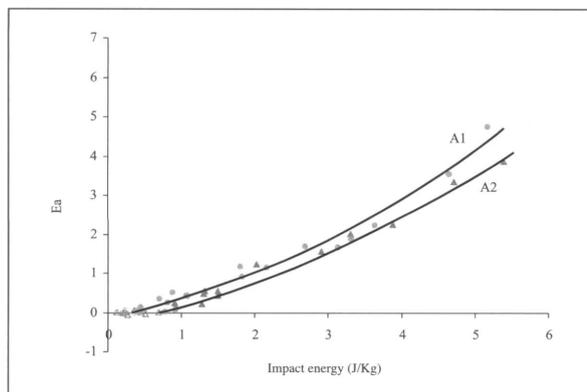
Figure 1. Impact test results of tiles A1 and A2.
